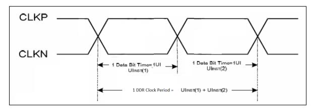
The same clock source is used to generate the DDR clock and launch the serial data. Since the clock and data signals propagate together over a channel of specified skew, the clock may be used directly to sample the date lines in the receiver. Such a system can accommodate large instantaneous variations in UI.
