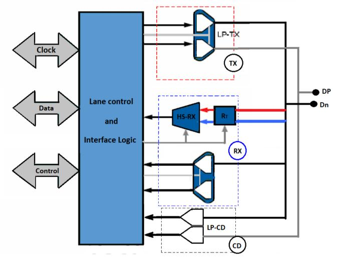
Where the HS receiver utilizes low-voltage swing differential signaling for signal transmission. The LP transmitter and LP receiver serve as a low power signaling mechanism. The figure shows both the HS and LP signal levels on the left and right sides, respectively. Because the HS signaling levels are below the LP low -level input threshold, the lane switches between low-power and high-speed mode during normal operation.
