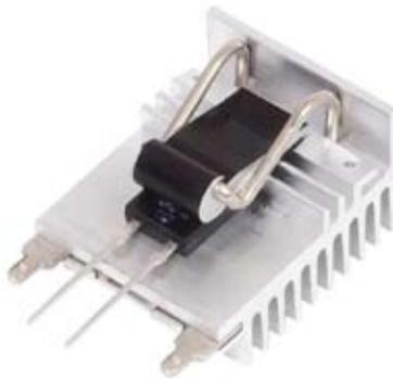
TNP10 resistors may be mounted with Ohmite **C Series (parts C126-XXX) heatsinks:**
