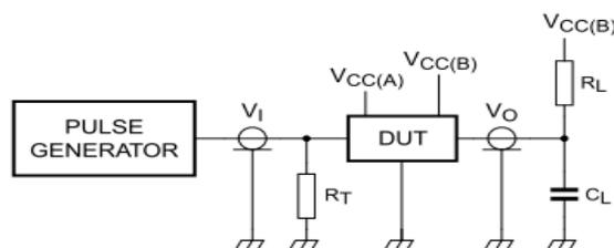
$R_L$  = Load resistor: 1.35k $\Omega$  on port B; 167 $\Omega$  on port A (0.8V to 2.7V) and 450 $\Omega$  on port A (3.0V to 5.5V)
