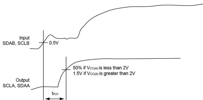
Figure 4: Propagation Delay
