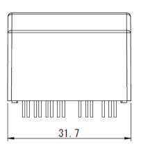
Note :1. The dimensional tolerance without directions is  $\pm$  0.5mm.
