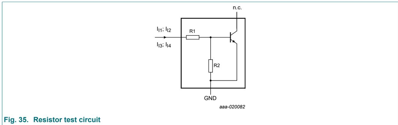
Fig. 35. Resistor test circuit
