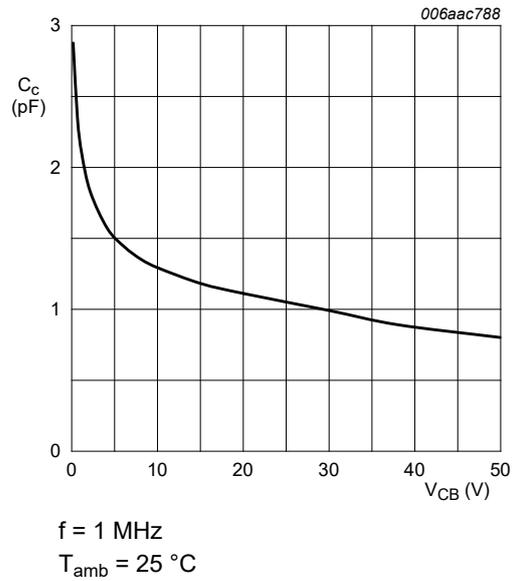
Fig. 27. PDTC114YQC: Collector capacitance as a function of collector-base voltage; typical values
