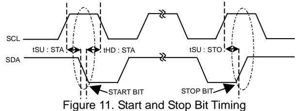
Figure 11. Start and Stop Bit Timing
