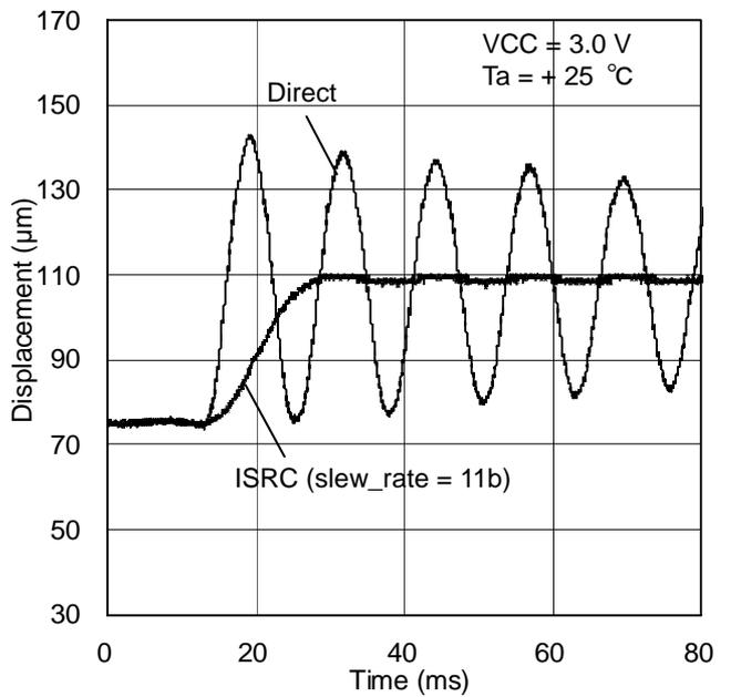
Figure 9. Displacement vs. settling time (slew\_rate = 11b)
