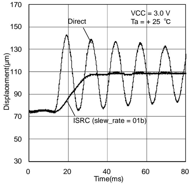
Figure 7. Displacement vs. settling time (slew\_rate = 01b)
