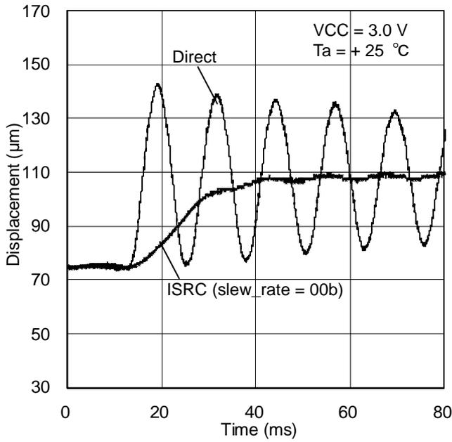
Figure 6. Displacement vs. settling time (slew\_rate = 00b)
