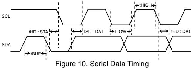
Figure 10. Serial Data Timing
