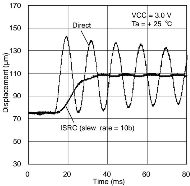
Figure 8. Displacement vs. settling time (slew\_rate = 10b)
