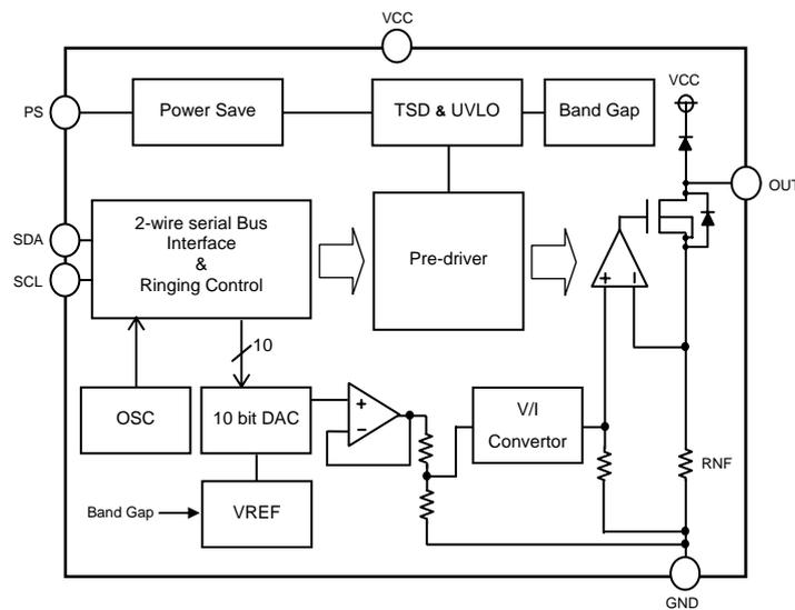
Figure 3. Block Diagram
