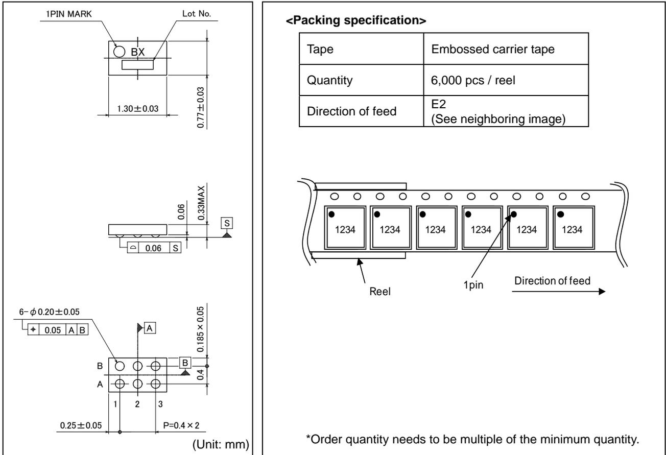
●Marking Diagram(TOP VIEW)
