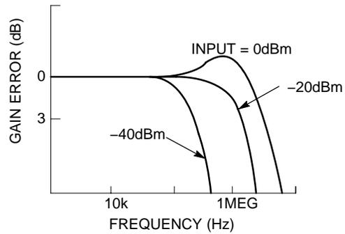
Figure 11. Rectifier Frequency Response vs. Input Level
