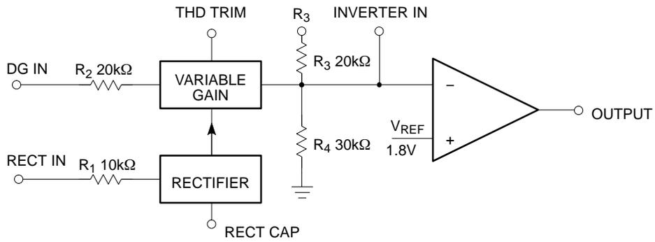
Figure 1. Block Diagram
