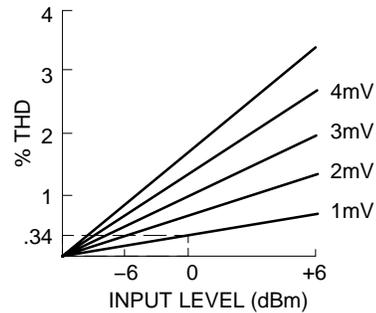
**Figure 13. ΔG Cell Distortion vs. Offset Voltage**
