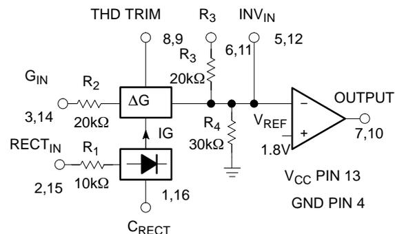
Figure 5. Chip Block Diagram (1 of 2 Channels)
