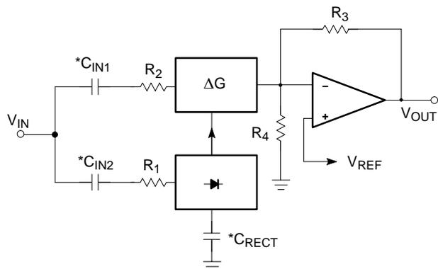
$$\text{NOTE: GAIN} = \left( \frac{2 R_3 V_{IN} (\text{avg})}{R_1 R_2 I_B} \right)^2$$
