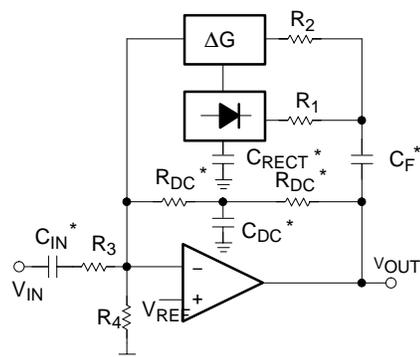
$$\text{NOTE: GAIN} = \left( \frac{R_1 R_2 I_B}{2 R_3 V_{IN \text{ avg}}} \right)^{\frac{1}{2}}$$
