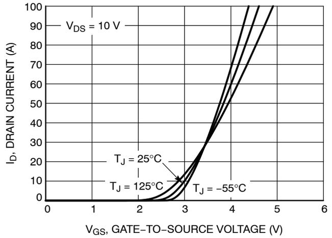
Figure 2. Transfer Characteristics
