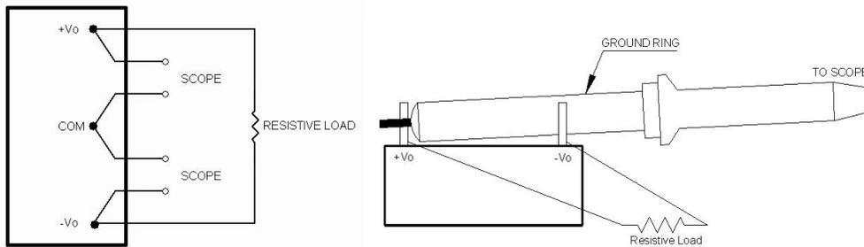
Output voltage and efficiency measurement test:
