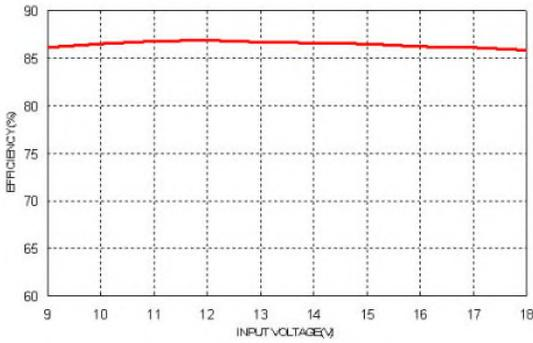
Efficiency Versus Input Voltage. Full Load
