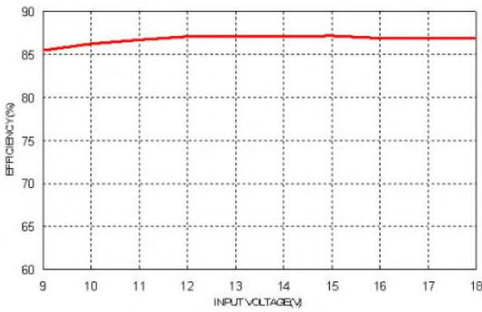
Efficiency Versus Input Voltage. Full Load
