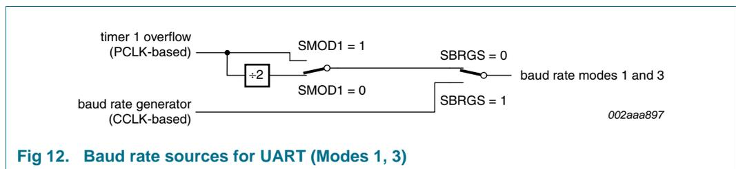
**Fig 12. Baud rate sources for UART (Modes 1, 3)**
