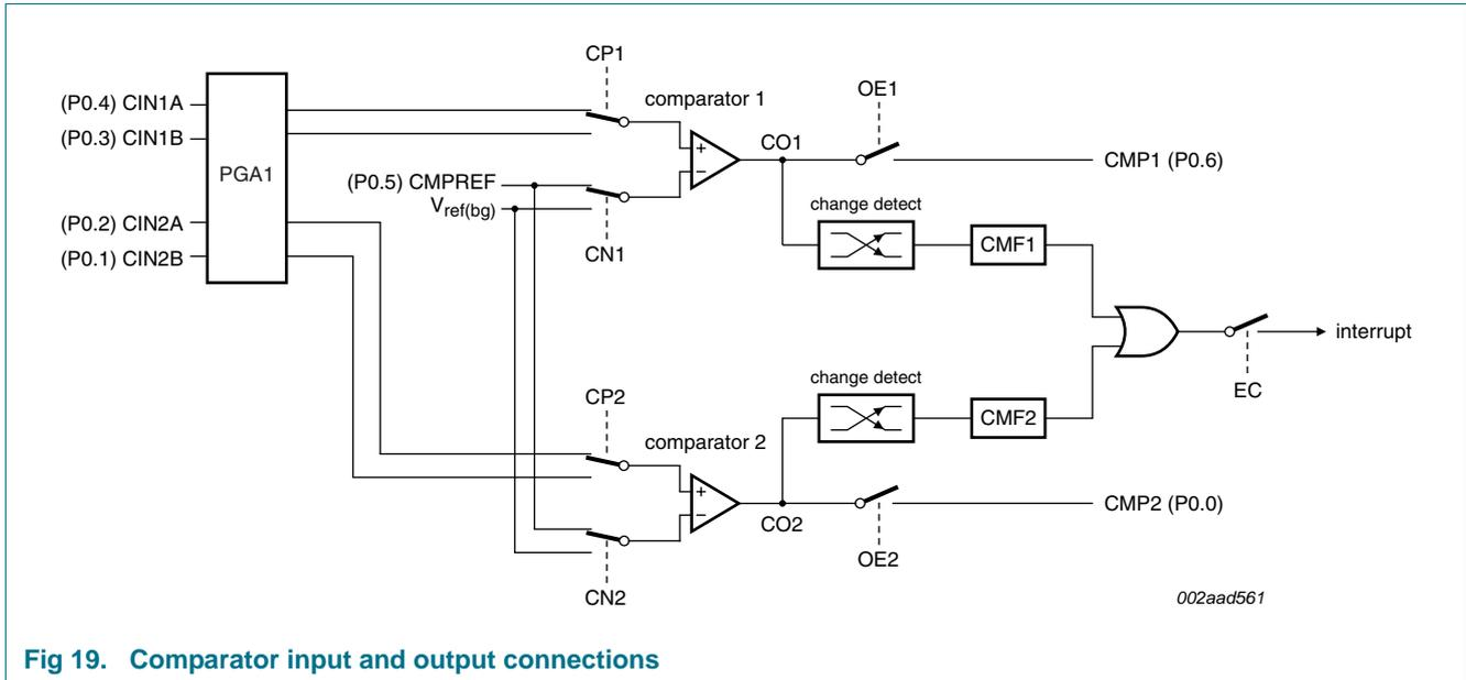
Fig 19. Comparator input and output connections
