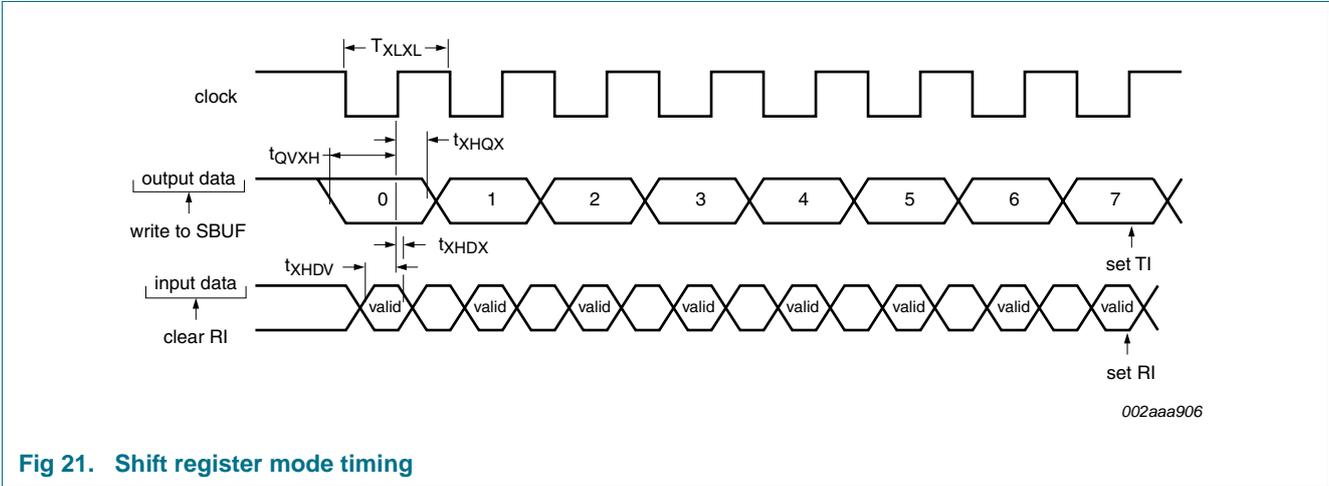
Fig 21. Shift register mode timing
