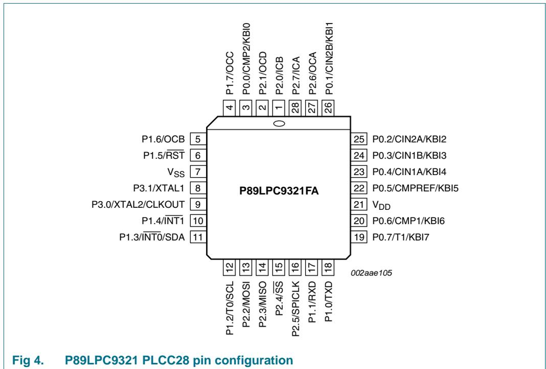
**Fig 4. P89LPC9321 PLCC28 pin configuration**
