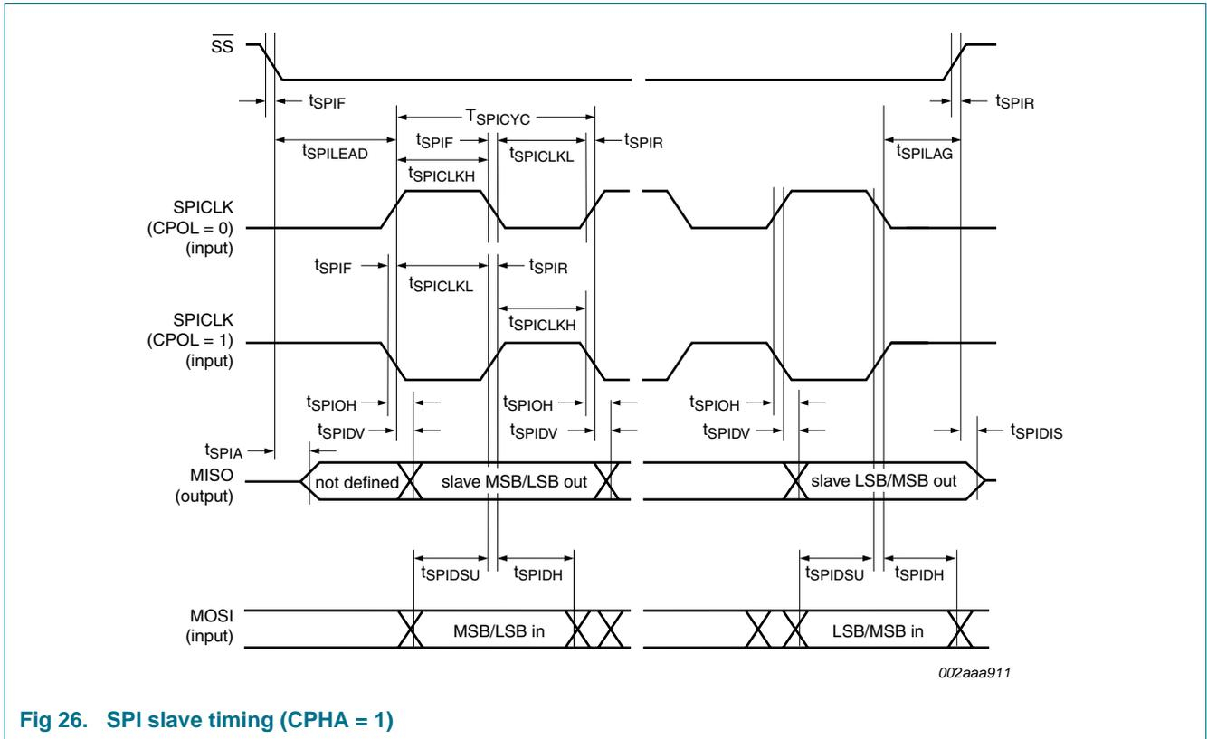
Fig 26. SPI slave timing (CPHA = 1)
