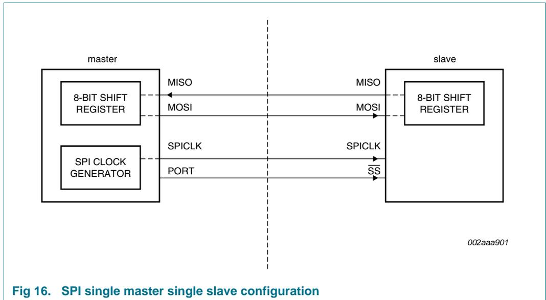
Fig 16. SPI single master single slave configuration
