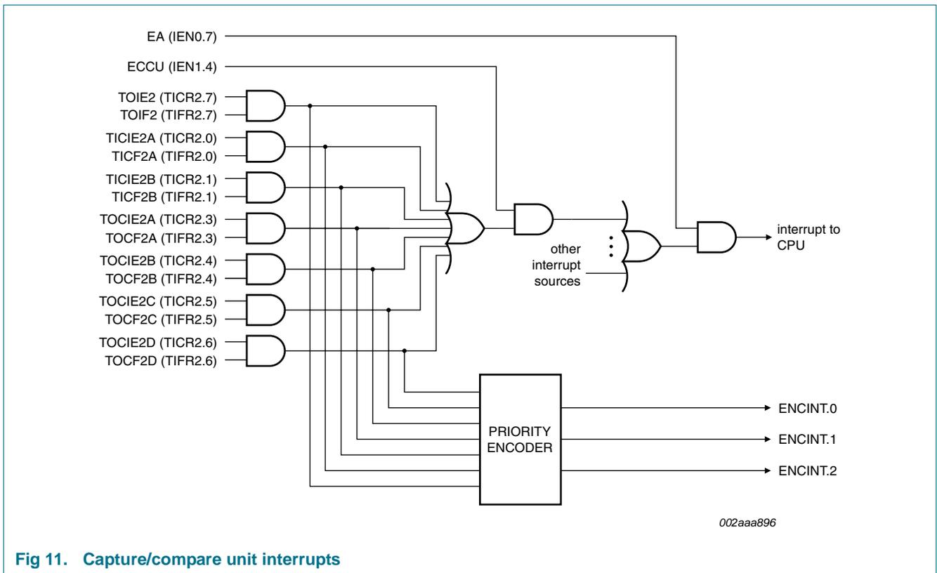
Fig 11. Capture/compare unit interrupts
