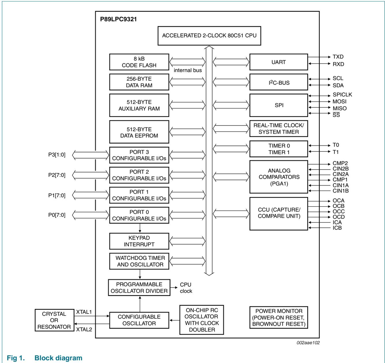
Fig 1. Block diagram
