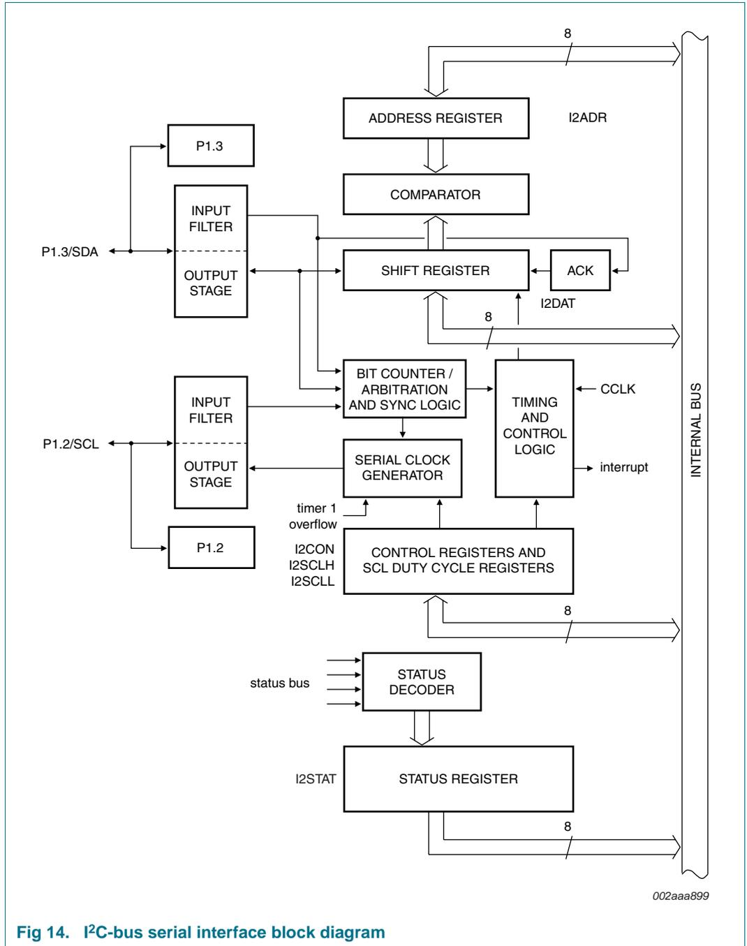
Fig 14. I<sup>2</sup>C-bus serial interface block diagram
