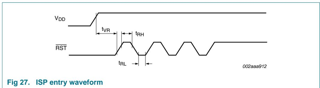
Fig 27. ISP entry waveform
