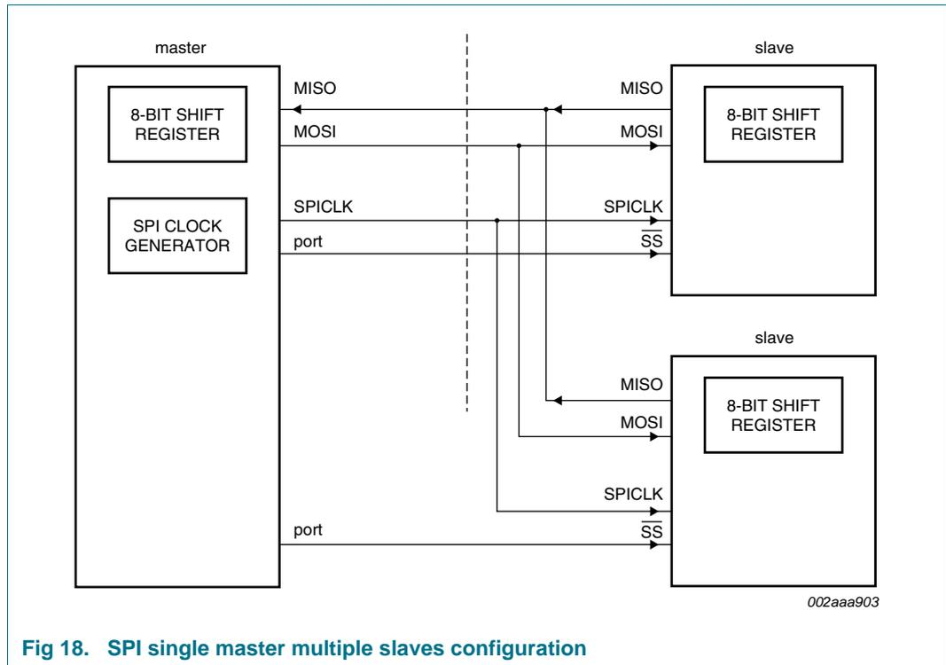
Fig 18. SPI single master multiple slaves configuration
