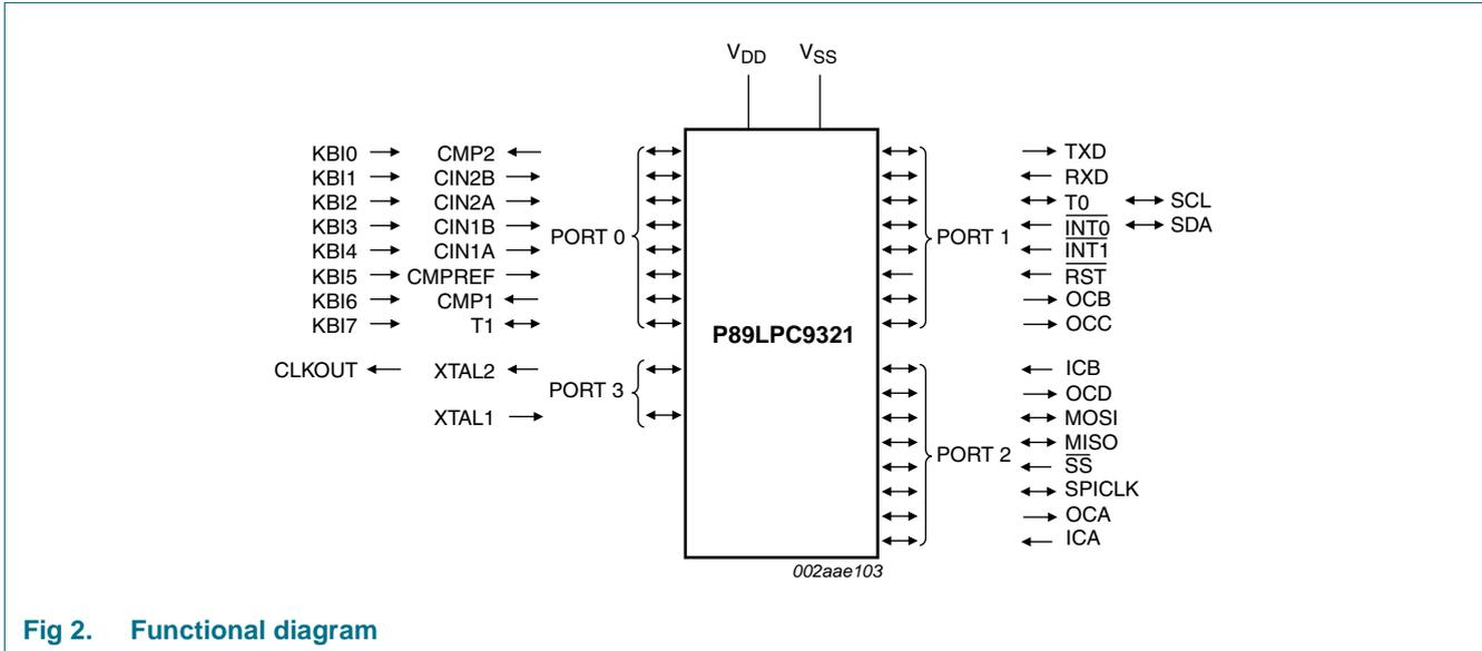
**Fig 2. Functional diagram**
