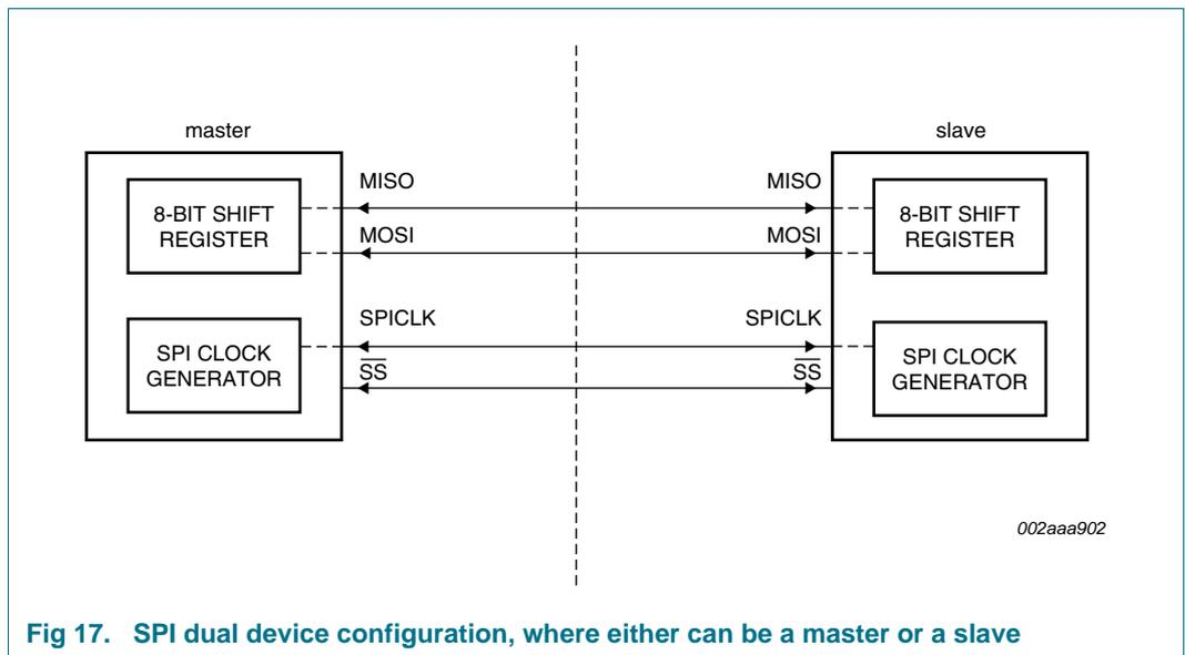
Fig 17. SPI dual device configuration, where either can be a master or a slave
