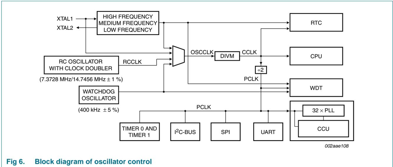
Fig 6. Block diagram of oscillator control
