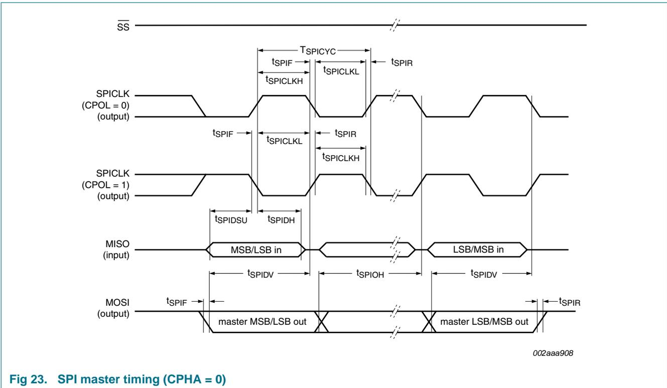
Fig 23. SPI master timing (CPHA = 0)
