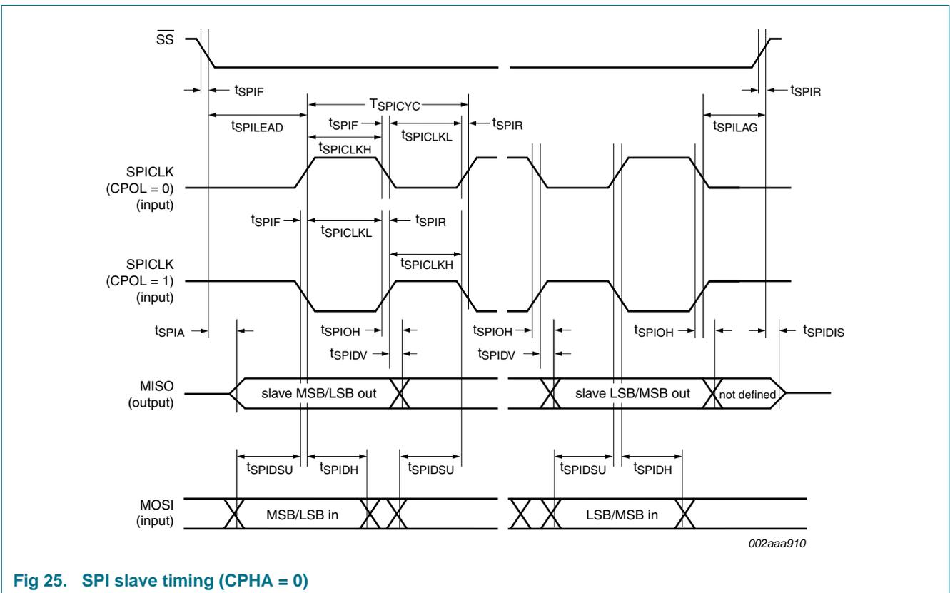
Fig 25. SPI slave timing (CPHA = 0)
