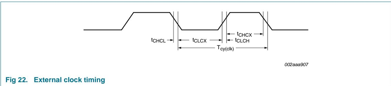
Fig 22. External clock timing
