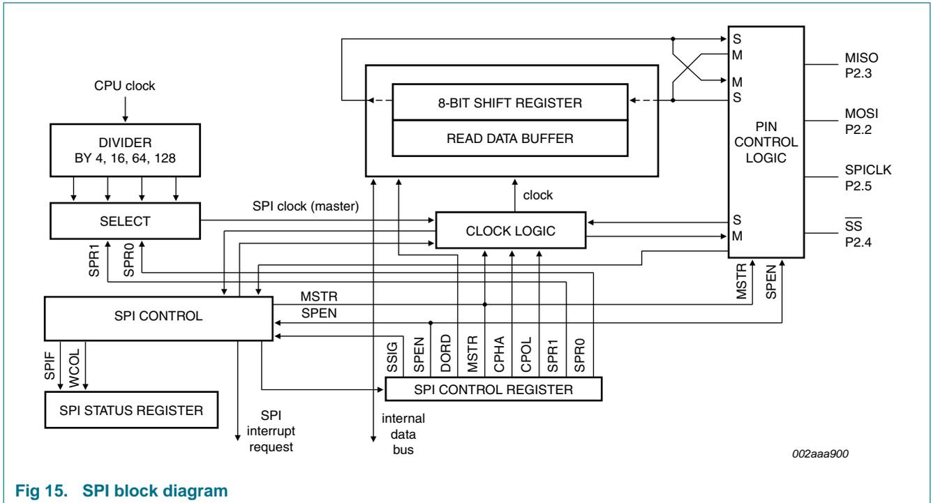
Fig 15. SPI block diagram
