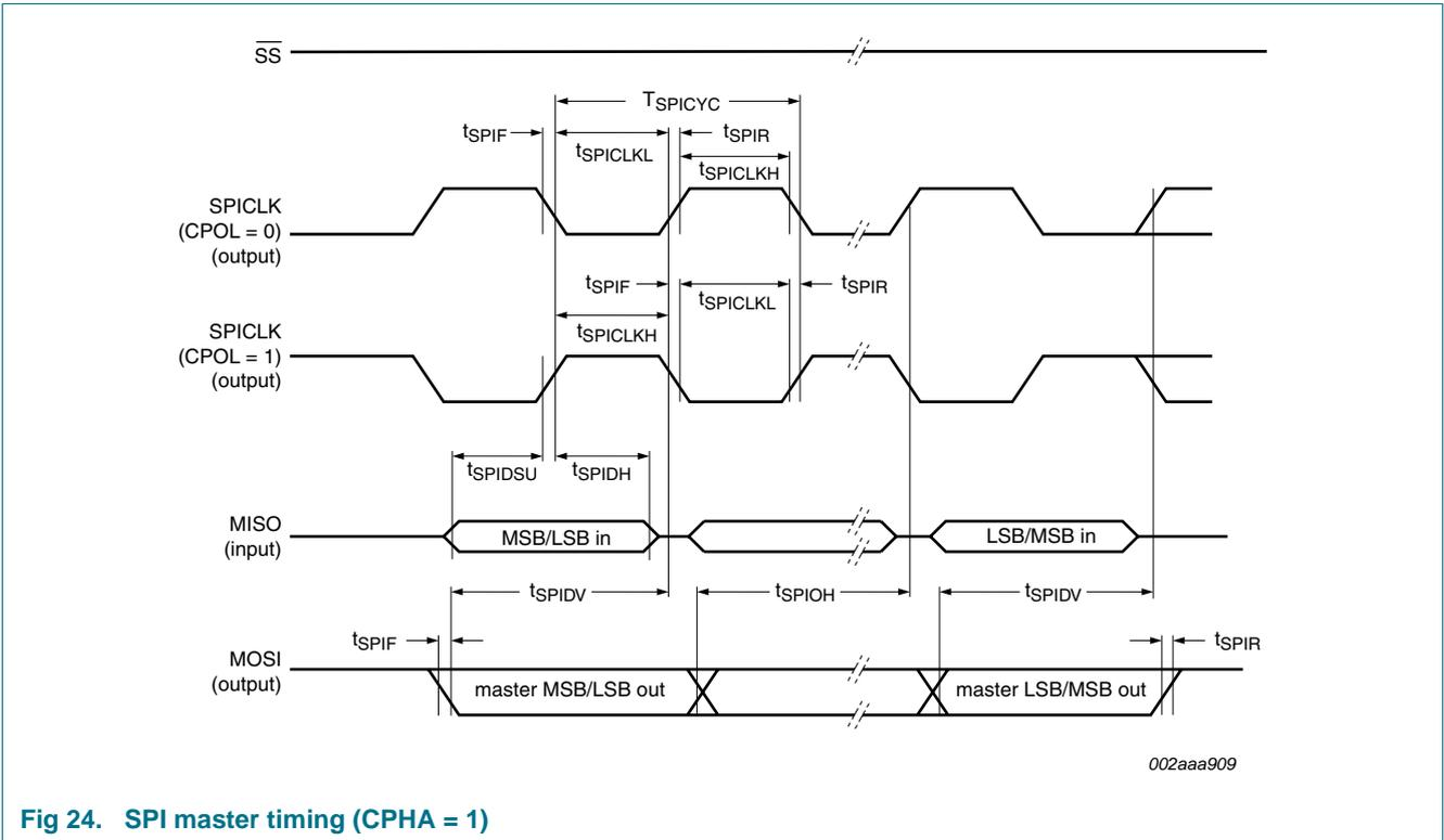
Fig 24. SPI master timing (CPHA = 1)
