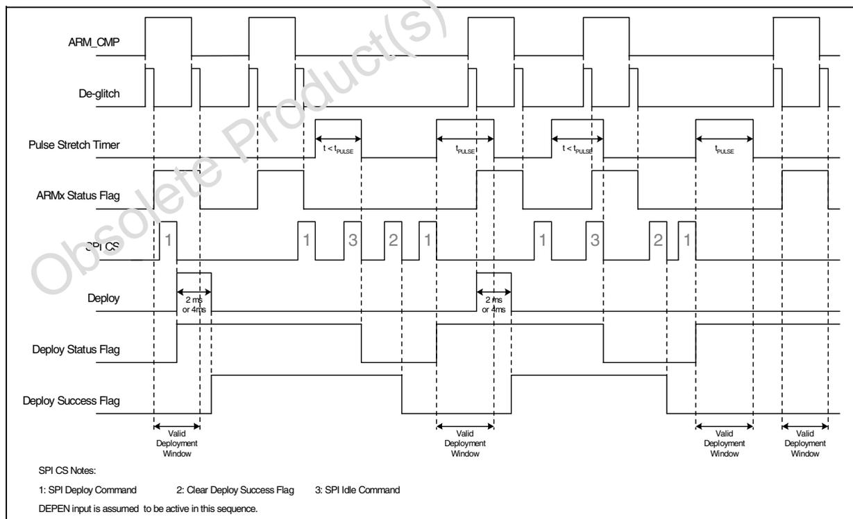
Figure 11. Serial Mode: Deployment Sequence with Pulse Stretch Timer Enabled
