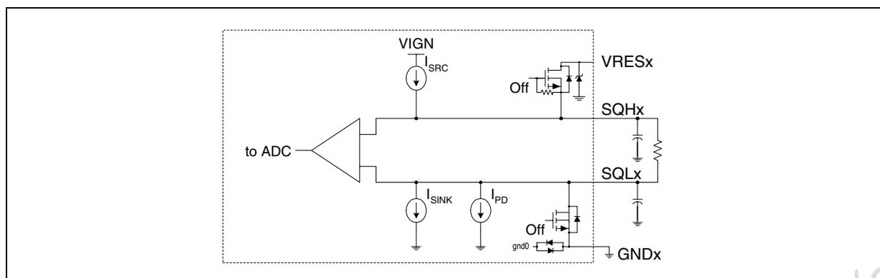
The ADC has a resolution of 8 bits and an accuracy of 5%. The ADC is robust to disruption that may occur due to adjacent loops short to 40V or -1V.
