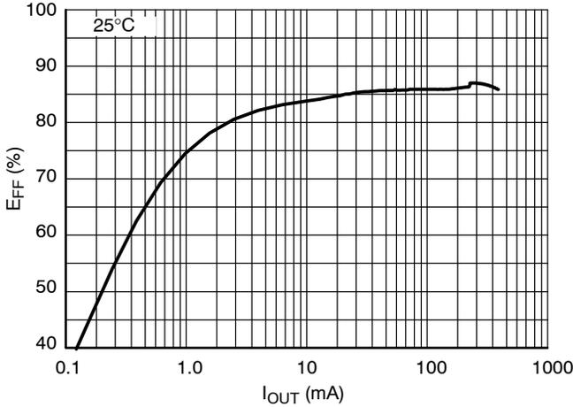
Figure 8. Efficiency versus IOUT (Auto Mode)
