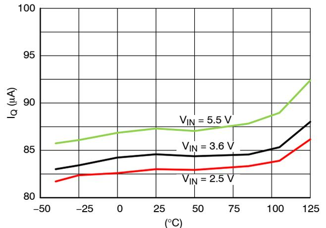
Figure 13. Quiescent Current versus Temperature,  $V_{\text{IN}}$  and  $PV_{\text{IN}}$  Tied Together HWEN High, LDOs on, DCDC On, No Switching
