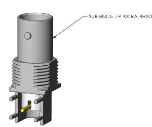
BNC5-J-P-XX-RA-BH2D **SERIES** BNC 50 OHM **TERMINATION** -BH2D: DIE CAST BULKHEAD THROUGH HOLE **GENDER** -J: JACK **ORIENTATION** -RA: RIGHT ANGLE -P: PCB PLATING SPECIFICATION -HN: HEAVY GOLD/NICKEL (SEE NOTES 3 & 4) (SUB-BNC5-J-P-HN-RA-BH2D) (BTNC-NUT-003-N) (BTNC-LWAS-001-N) -GN: GOLD/NICKEL (SEE NOTES 3 & 4) (SUB-BNC5-J-P-GN-RA-BH2D) (BTNC-NUT-003-N) (BTNC-LWAS-001-N)
