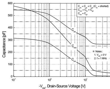
**Figure 5. Capacitance Characteristics**
