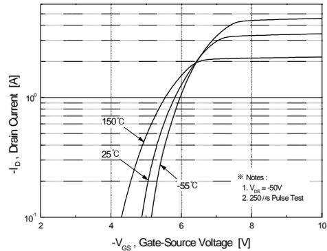
**Figure 2. Transfer Characteristics**
