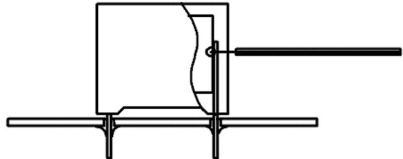
*Temperature monitored inside the capacitor.*
