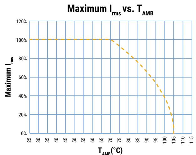
$T_{AMB}$  is the maximum ambient temperature surrounding the capacitor or hottest contact point (e.g. tracks), whichever is higher, in the worst operation conditions in °C.
