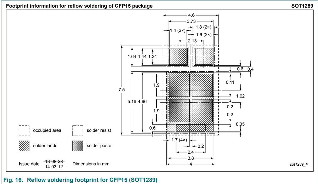
Fig. 16. Reflow soldering footprint for CFP15 (SOT1289)
