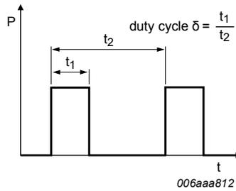
Fig. 14. Duty cycle definition
