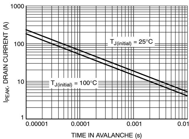
Figure 12. Maximum Drain Current vs. Time in Avalanche
