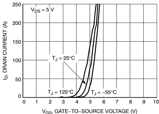
Figure 2. Transfer Characteristics
