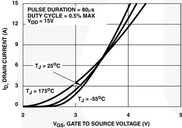
FIGURE 7. TRANSFER CHARACTERISTICS
