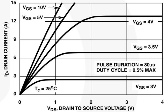
FIGURE 8. SATURATION CHARACTERISTICS
