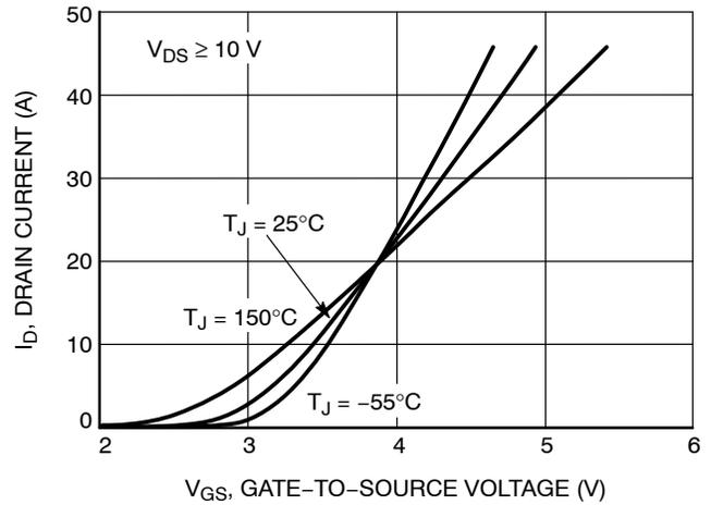
Figure 2. Transfer Characteristics
