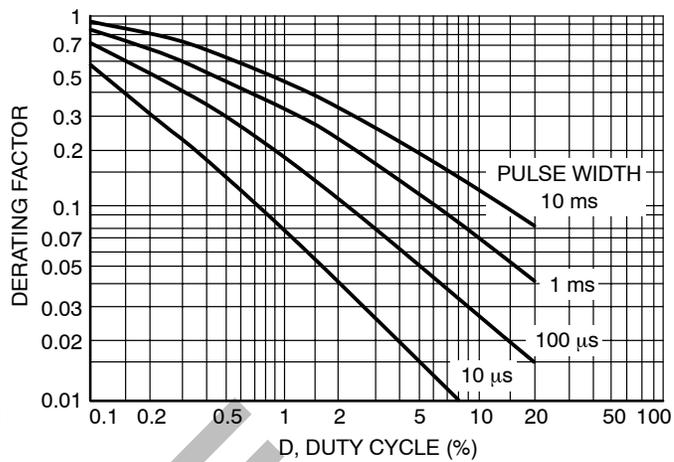
**Figure 4. Typical Derating Factor for Duty Cycle**
