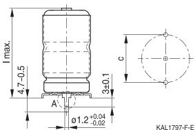
Soldering star capacitors, 2-pin design
