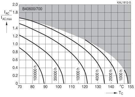
\*) Maximum ripple current I<sub>AC</sub> under continous operation is limited to 35 A.
