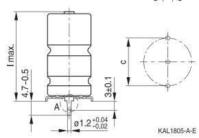
Soldering star capacitors, 2-pin design
