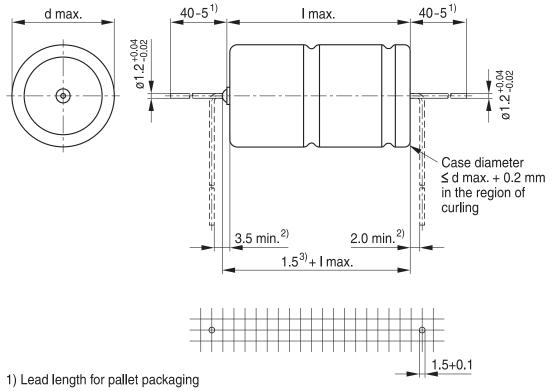
2) Minimum bending distance recommended per wire
