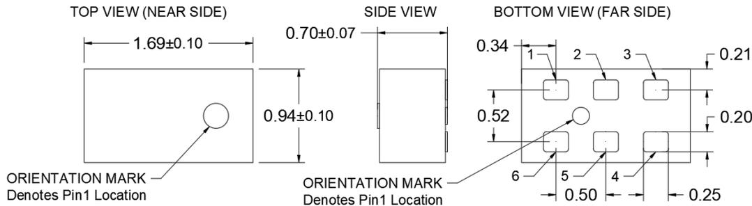
Dimensions are in Millimeters
