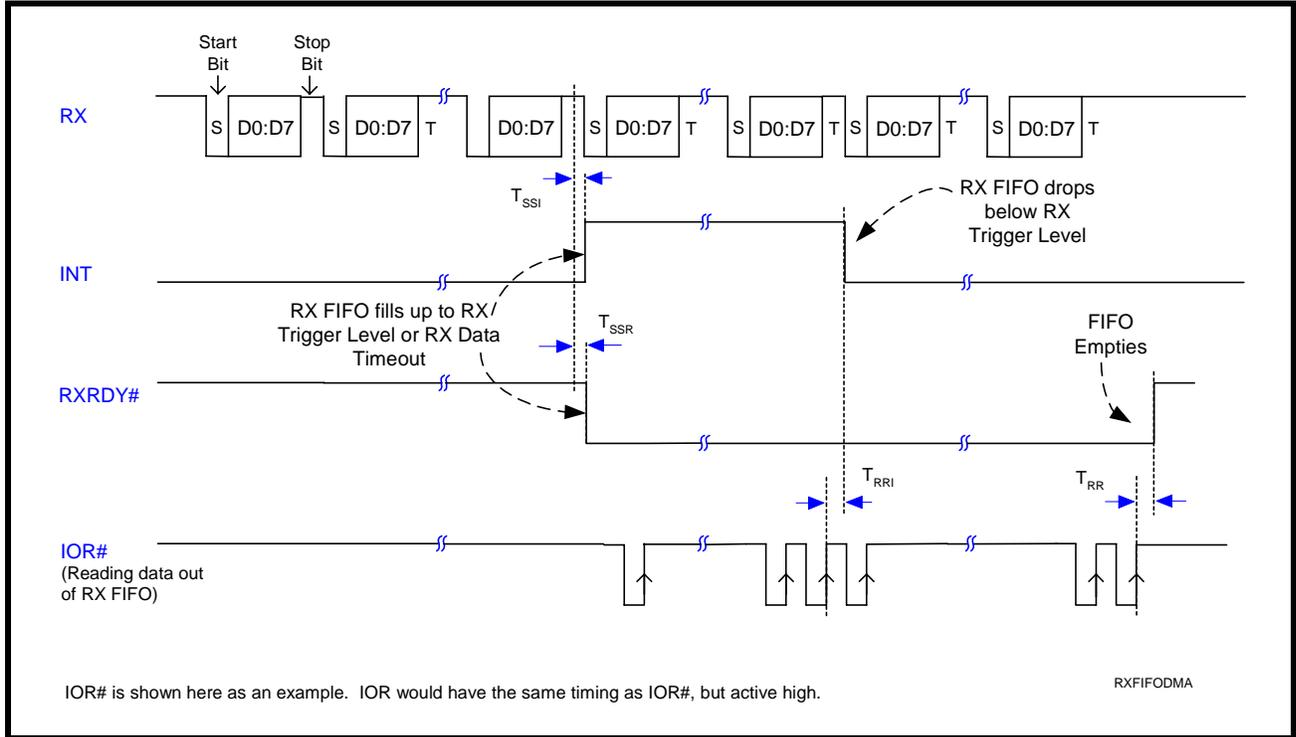
**FIGURE 30. TRANSMIT READY & INTERRUPT TIMING [FIFO MODE, DMA MODE DISABLED]**
