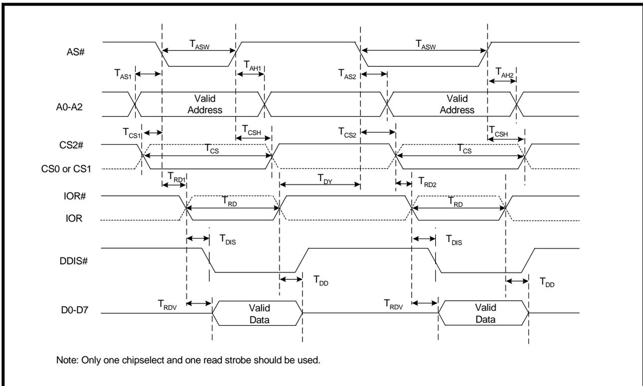
**FIGURE 21. 16 MODE (INTEL) DATA BUS WRITE TIMING USING AS#**
