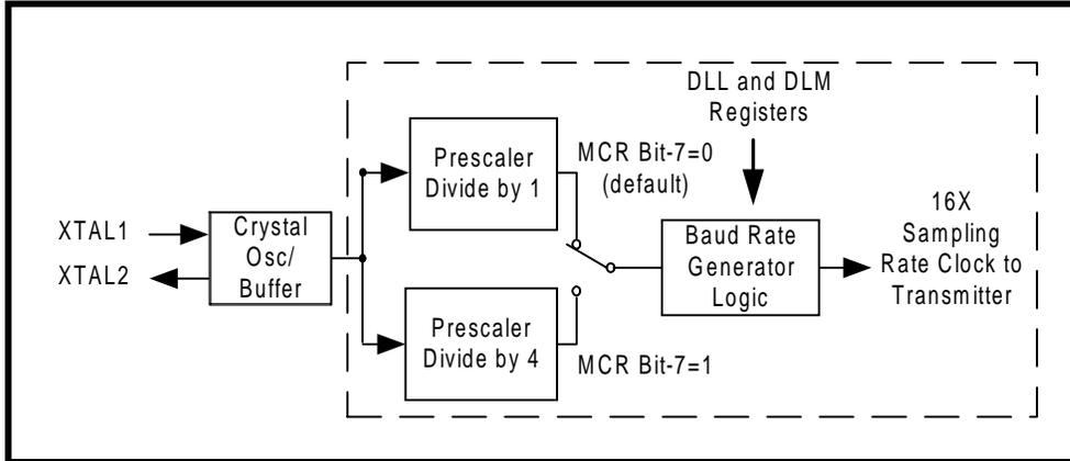
Programming the Baud Rate Generator Registers DLM and DLL provides the capability of selecting the operating data rate. Table 4 shows the standard data rates available with a 14.7456 MHz crystal or external clock at 16X clock rate. When using a non-standard data rate crystal or external clock, the divisor value can be calculated for DLL/DLM with the following equation.
