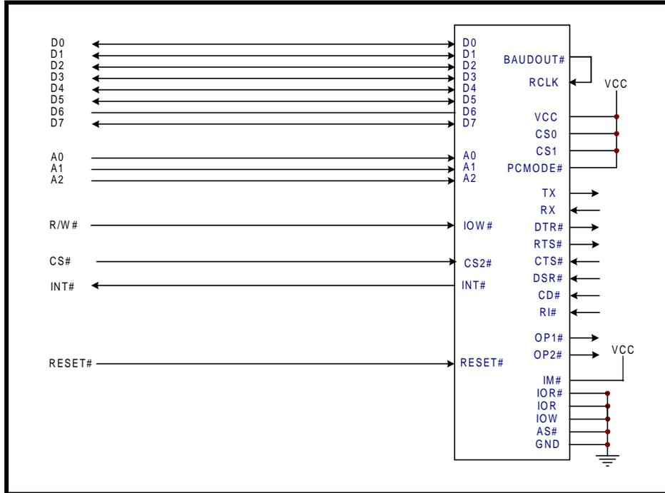
**FIGURE 5. XR16L651 PC MODE INTERCONNECTIONS**
