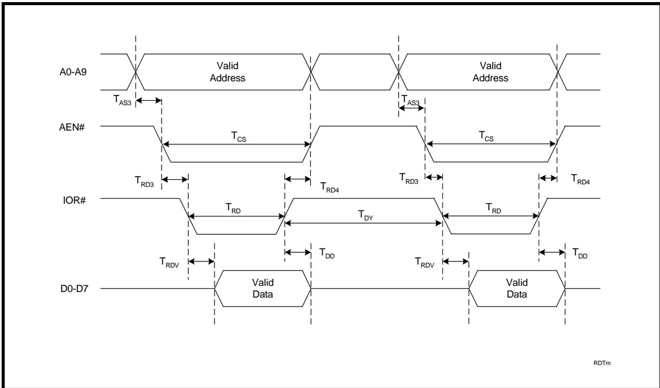
**FIGURE 25. DATA BUS WRITE TIMING IN PC MODE**
