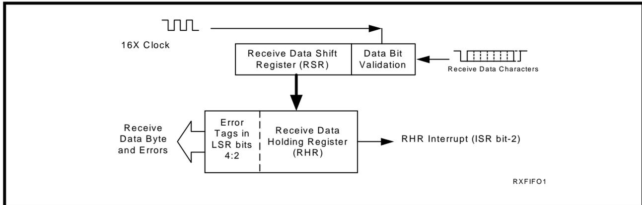
**FIGURE 12. RECEIVER OPERATION IN FIFO AND AUTO RTS FLOW CONTROL MODE**
