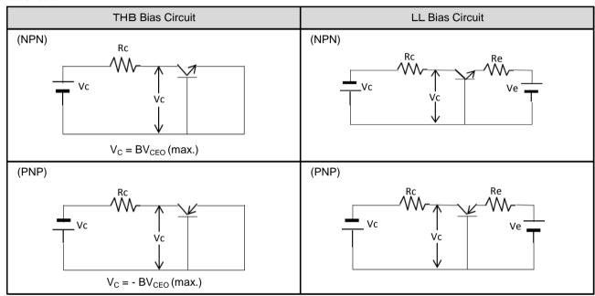
Built-in resistor of digital transistors omitted
