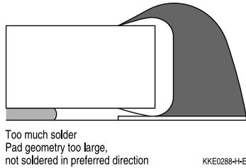
Good and poor solder joints caused by amount of solder in dual-wave soldering.
