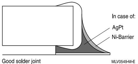
Good and poor solder joints caused by amount of solder in reflow soldering.
