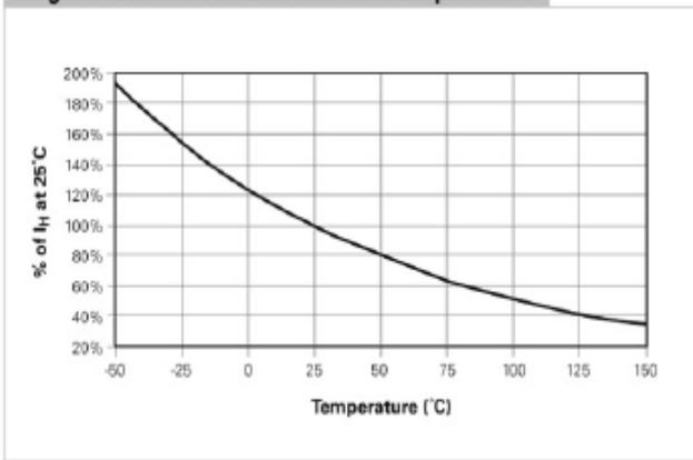
**Figure SB6 - Off-state Current vs. Temperature**
