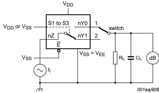
Fig. 18. Test circuit for measuring isolation (OFF-state)
