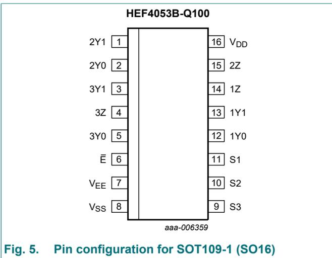
Fig. 5. Pin configuration for SOT109-1 (SO16)
