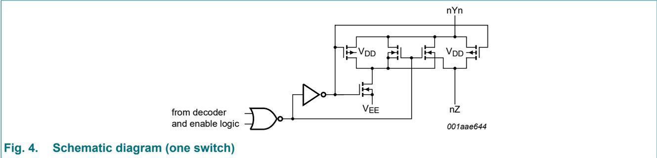
Fig. 4. Schematic diagram (one switch)
