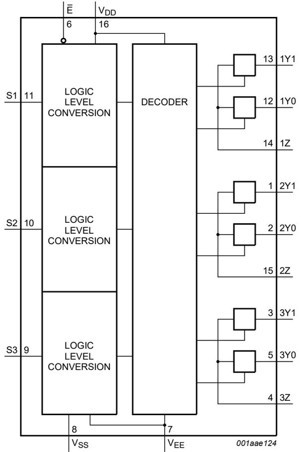
Fig. 2. Functional diagram
