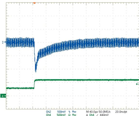
Step Load Transient Response (Vin=12V, Vout=5.0V, Load=0, Iout=3A to 1.5A)
