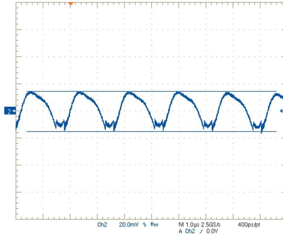
Step Load Transient Response (Vin=12V, Vout=1.8V, Cload=0, Iout=1.5A to 3A)
