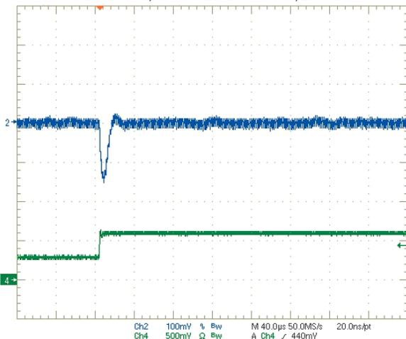
Step Load Transient Response (Vin=12V, Vout=1.2V, Clod=0, Iout=3A to 1.5A)
