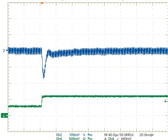
Step Load Transient Response (Vin=12V, Vout=2.5V, Cloud=0, Iout=3A to 1.5A)
