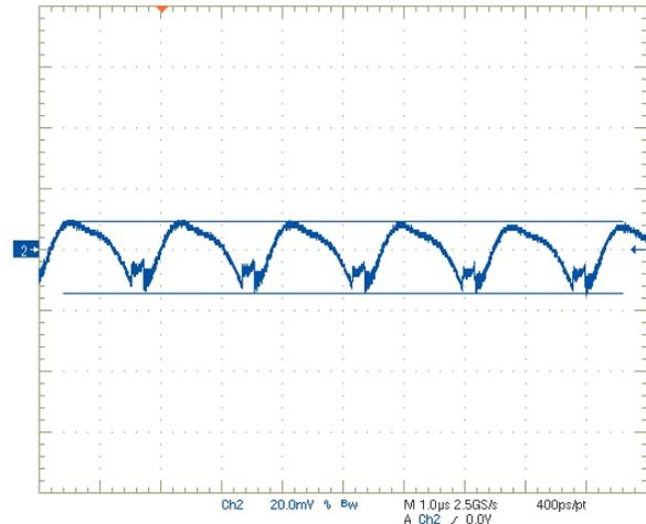
Step Load Transient Response (Vin=12V, Vout=1.2V, Clod=0, Iout=1.5A to 3A)
