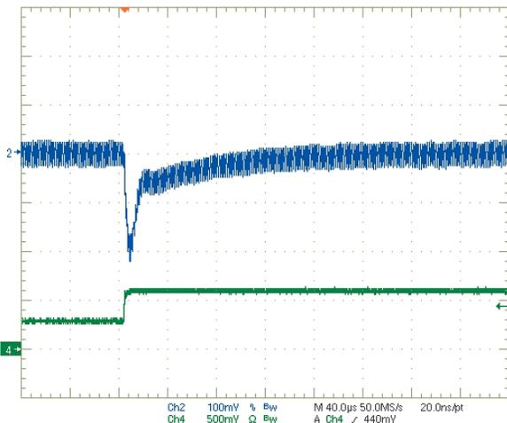
Step Load Transient Response (Vin=12V, Vout=3.3V, Cload=0, Iout=3A to 1.5A)
