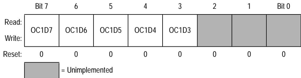
**Figure 9-14. Output Compare 1 Data Register (OC1D)**
