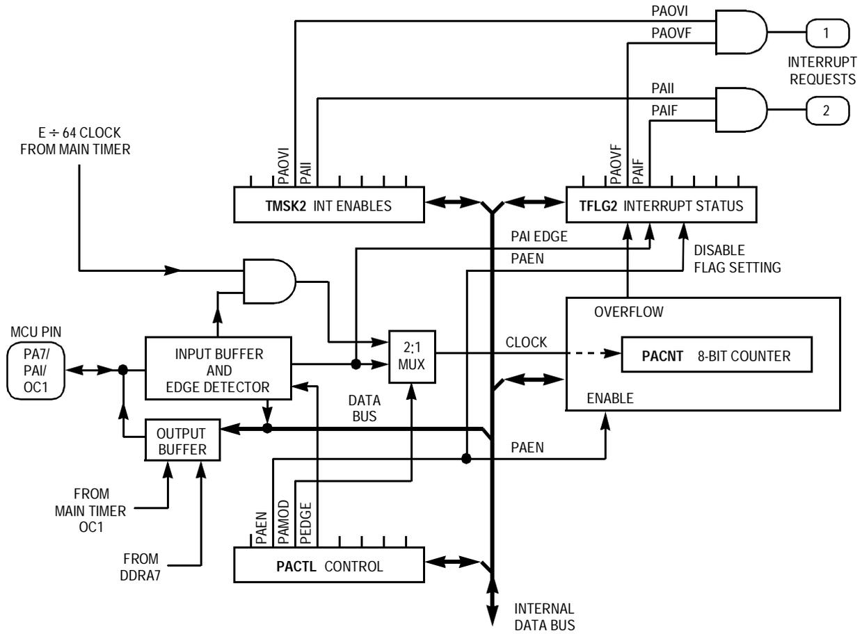
**Figure 9-24. Pulse Accumulator**
