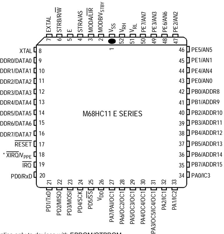
**Figure 2-1. Pin Assignments for 52-Pin PLCC and CLCC**
