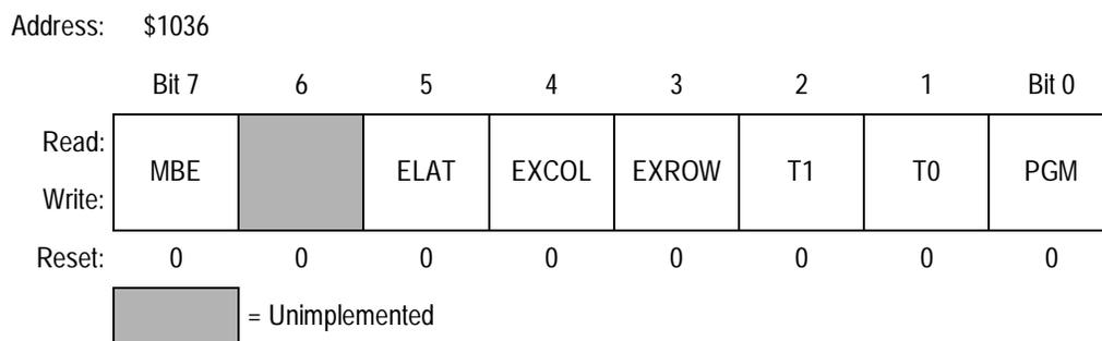
**Figure 4-15. MC68HC711E20 EPROM Programming Control Register (EPROG)**
