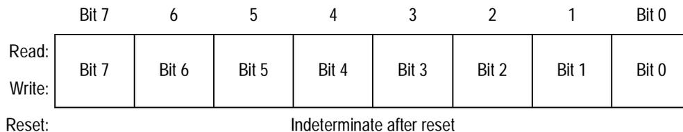
**Figure 8-5. Serial Peripheral Data I/O Register (SPDR)**
