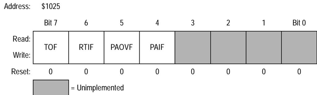
**Figure 9-22. Timer Interrupt Flag 2 Register (TFLG2)**
