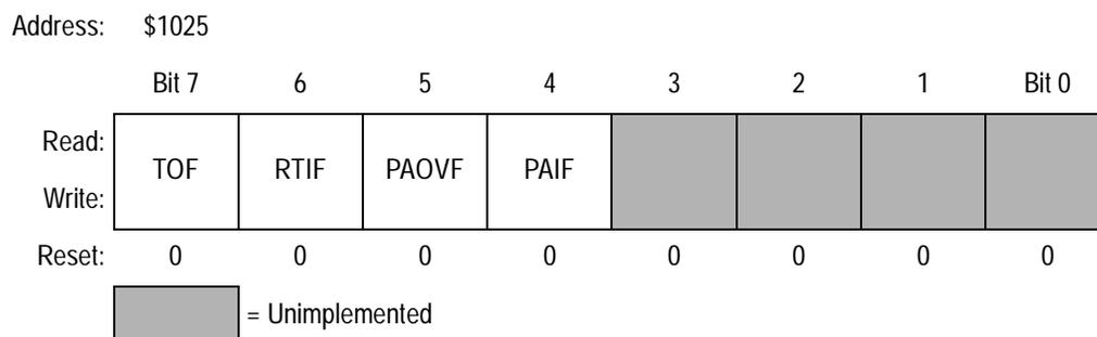
**Figure 9-28. Timer Interrupt Flag 2 Register (TFLG2)**
