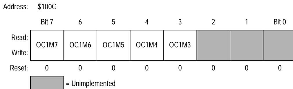
**Figure 9-13. Output Compare 1 Mask Register (OC1M)**
