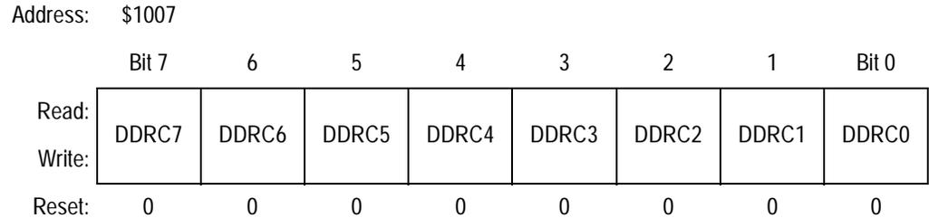
**Figure 6-6. Port C Data Direction Register (DDRC)**
