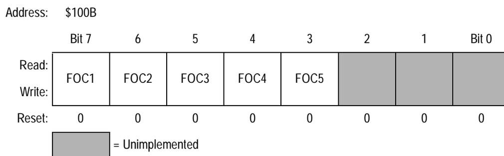
**Figure 9-12. Timer Compare Force Register (CFORC)**
