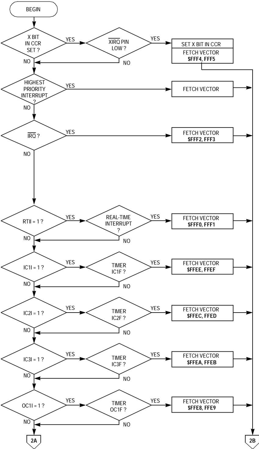
Figure 5-6. Interrupt Priority Resolution (Sheet 1 of 2)
