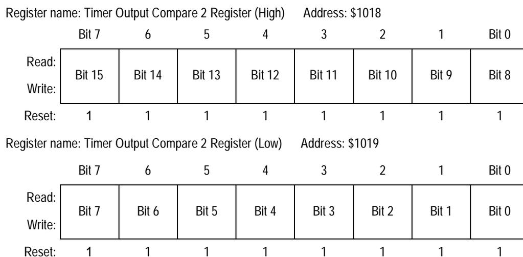
**Figure 9-9. Timer Output Compare 2 Register Pair (TOC2)**
