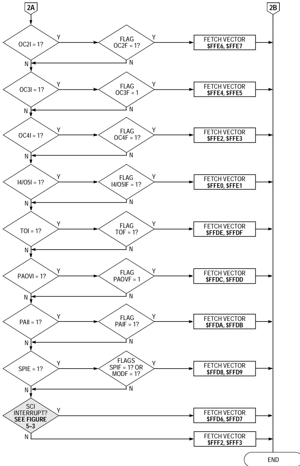
**Figure 5-6. Interrupt Priority Resolution (Sheet 2 of 2)**
