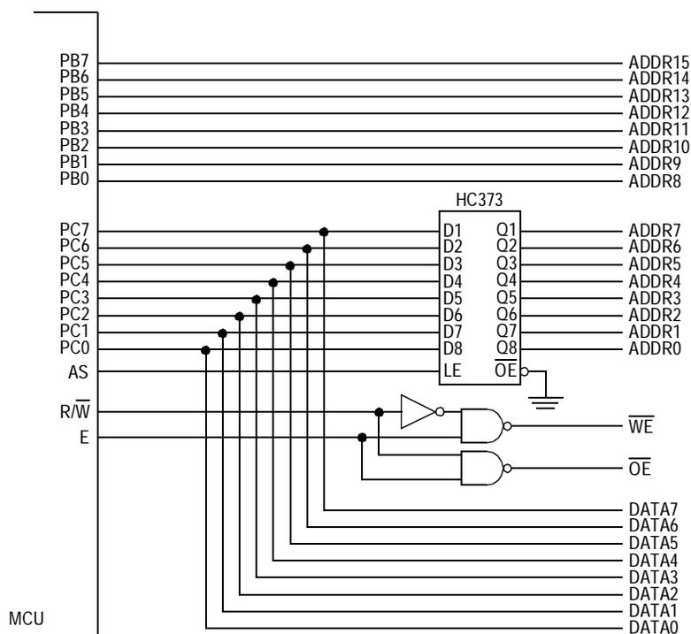
**Figure 4-1. Address/Data Demultiplexing**
