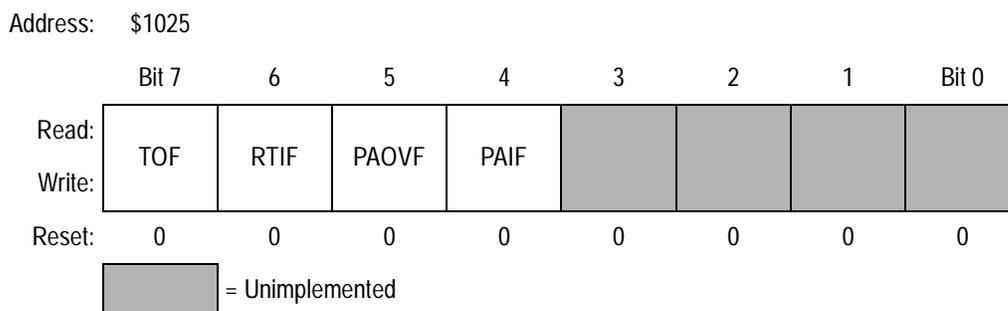
**Figure 9-20. Timer Interrupt Flag 2 Register (TFLG2)**
