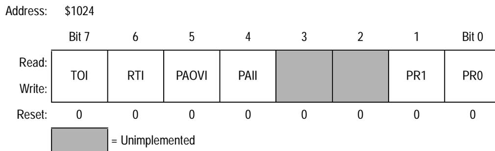
**Figure 9-21. Timer Interrupt Mask 2 Register (TMSK2)**
