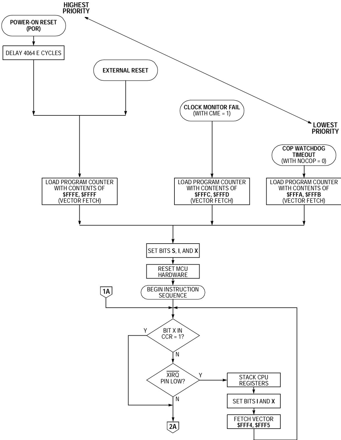
Figure 5-5. Processing Flow Out of Reset (Sheet 1 of 2)
