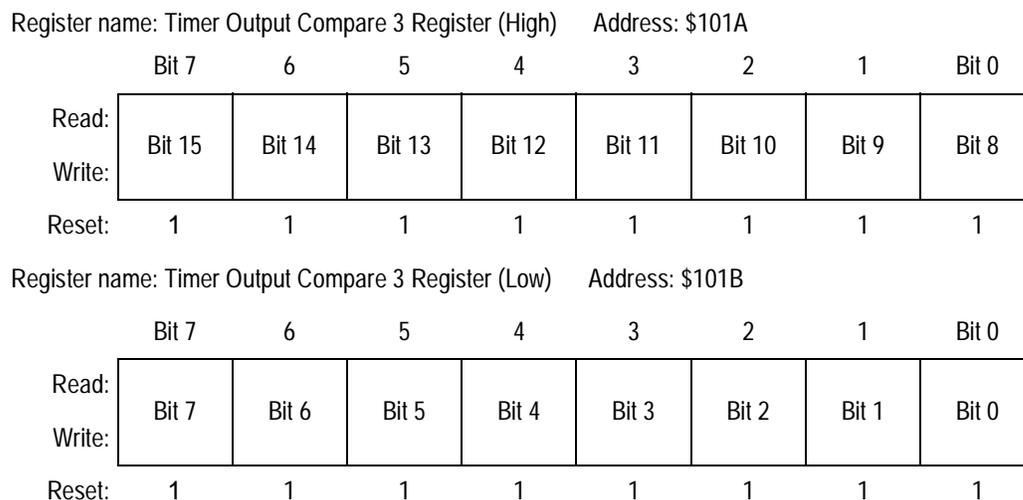
**Figure 9-10. Timer Output Compare 3 Register Pair (TOC3)**
