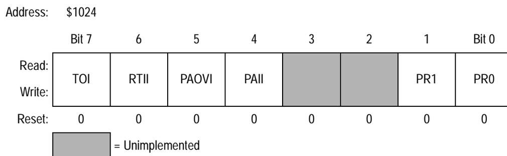
**Figure 9-27. Timer Interrupt Mask 2 Register (TMSK2)**
