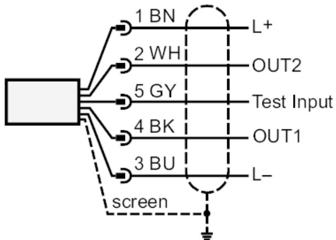
OUT1: switching output / IO-Link
