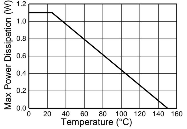
Figure 2. Derating Curve
