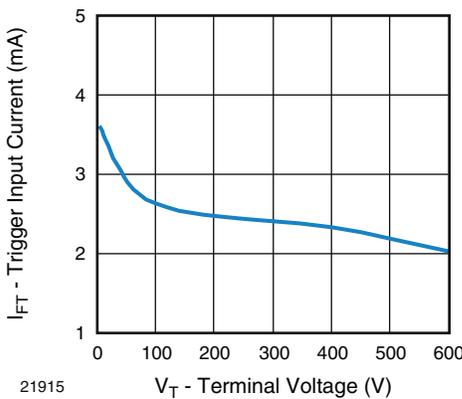
Fig. 12 - Trigger Current vs. V<sub>LOAD</sub>
