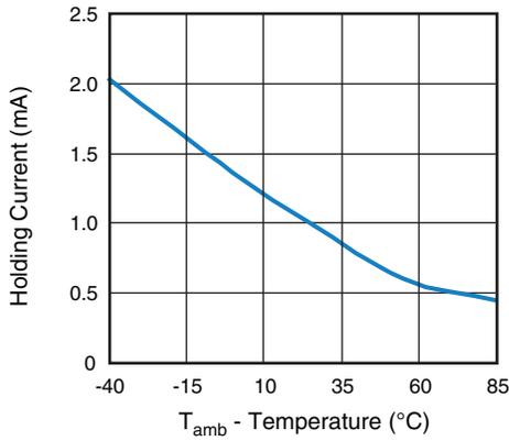
Fig. 10 - Normalized Holding Current vs. Temperature
