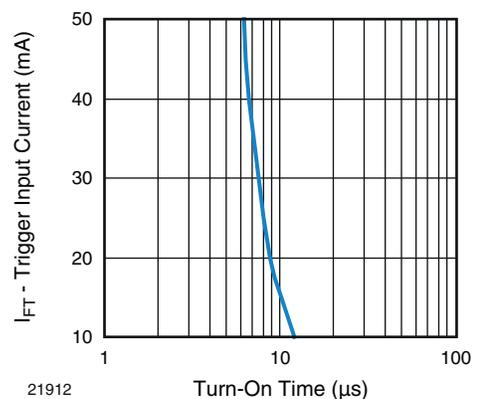
Fig. 9 - Trigger Input Current vs. Turn-on Time
