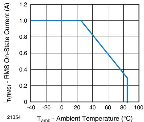
Fig. 2 - Allowable Load Current vs. Ambient Temperature
