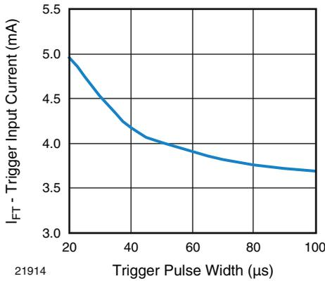
Fig. 11 - Trigger Current vs. Trigger Pulse Width
