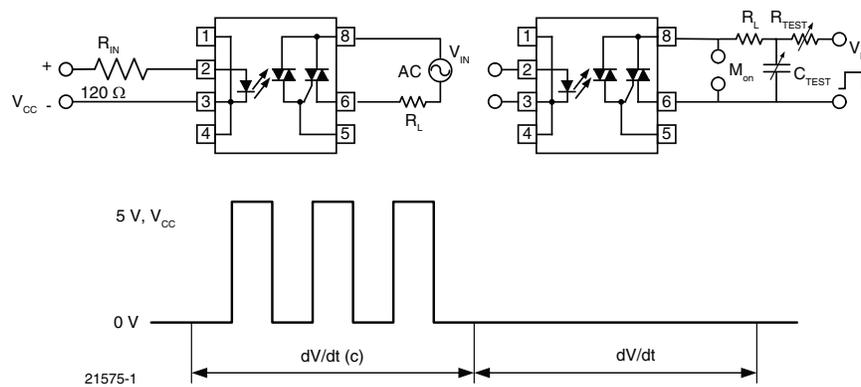
Fig. 3 - dV/dt Test Circuit
