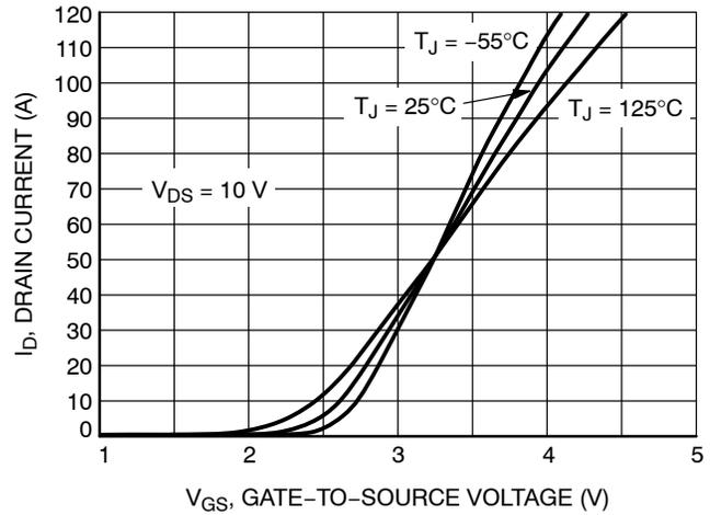
Figure 2. Transfer Characteristics
