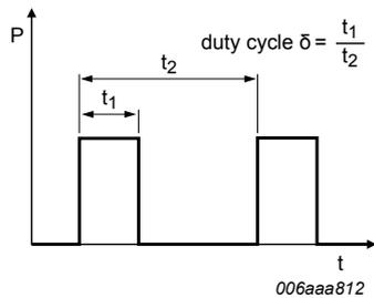
Fig. 17. Duty cycle definition
