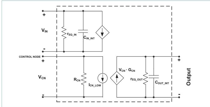
Figure 24 — PRM48BH480x250A00 AC small signal model
