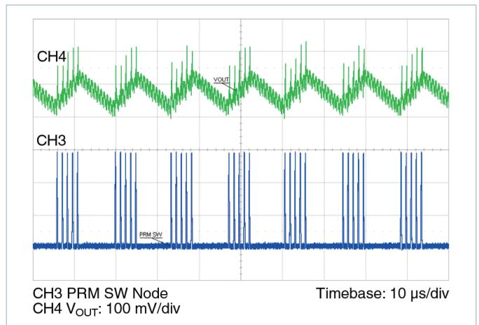
**Figure 41** — Light load burst mode of operation
