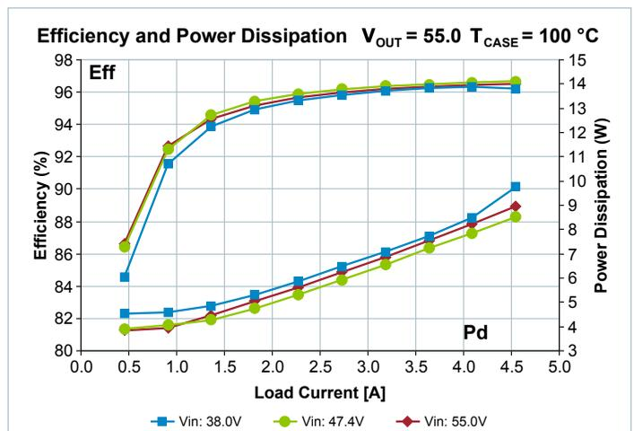
Figure 12 — Total efficiency and power dissipation vs.  $V_{IN}$  and  $I_{OUT}$
