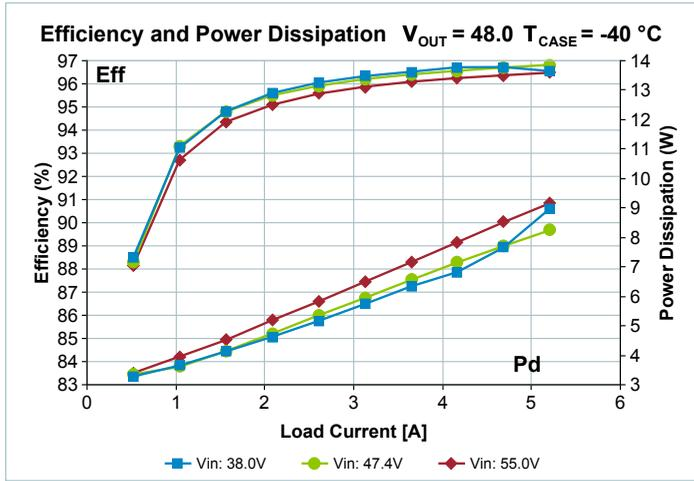
Figure 7 — Total efficiency and power dissipation vs.  $V_{IN}$  and  $I_{OUT}$
