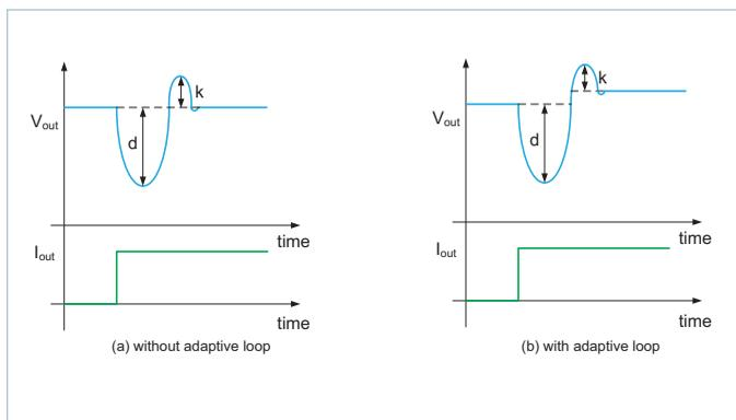
**Figure 40** — Load step response example and “droop” vs. “kick”
