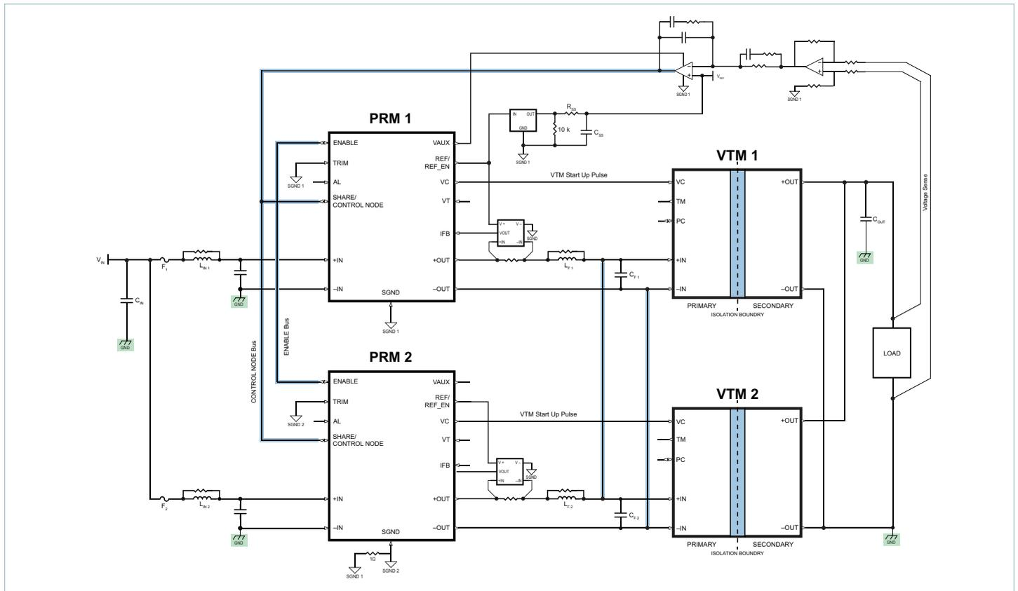
Figure 39 — Non-Isolated Remote Sense Array Example
