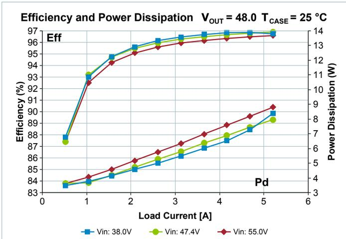
Figure 8 — Total efficiency and power dissipation vs.  $V_{IN}$  and  $I_{OUT}$
