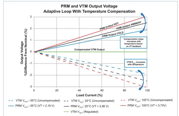
Figure 31 — Adaptive Loop Temperature Compensation Illustration
