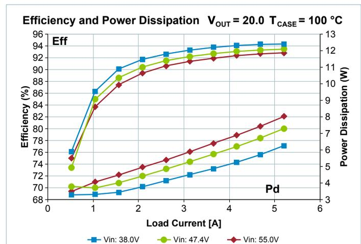
Figure 6 — Total efficiency and power dissipation vs.  $V_{IN}$  and  $I_{OUT}$
