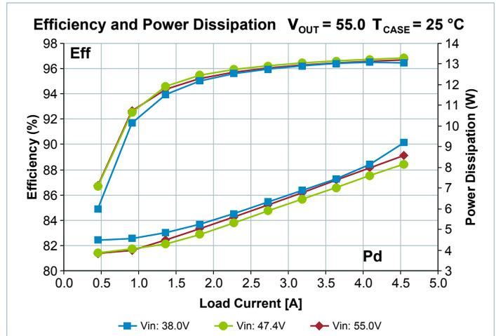
Figure 11 — Total efficiency and power dissipation vs.  $V_{IN}$  and  $I_{OUT}$
