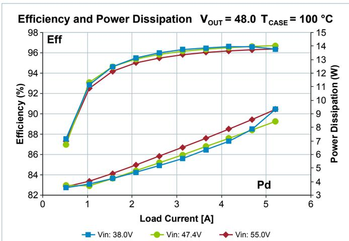
Figure 9 — Total efficiency and power dissipation vs.  $V_{IN}$  and  $I_{OUT}$
