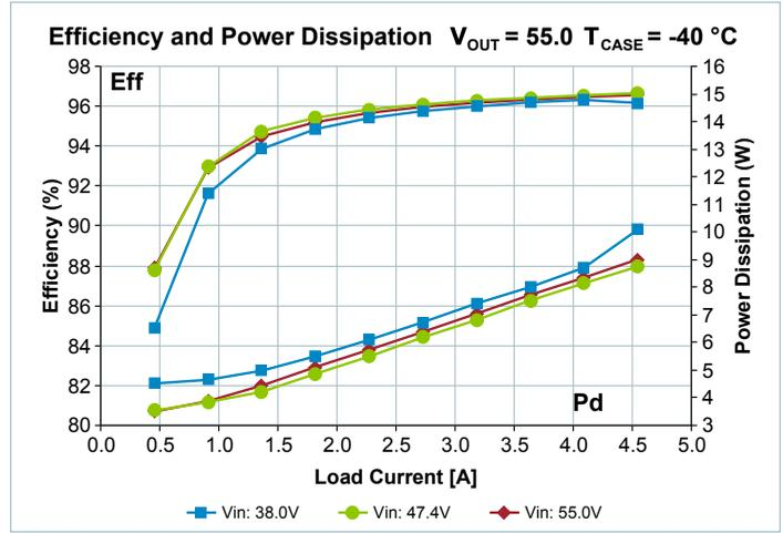
Figure 10 — Total efficiency and power dissipation vs.  $V_{IN}$  and  $I_{OUT}$
