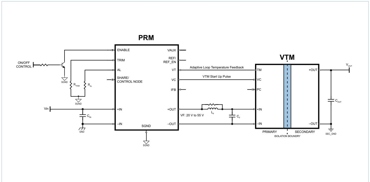
Typical Application: PRM48BH480x250A00 + VTM Adaptive Loop Configuration
