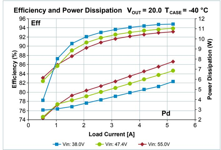
Figure 4 — Total efficiency and power dissipation vs.  $V_{IN}$  and  $I_{OUT}$
