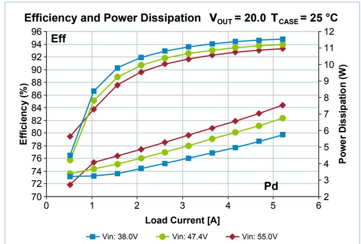
Figure 5 — Total efficiency and power dissipation vs.  $V_{IN}$  and  $I_{OUT}$
