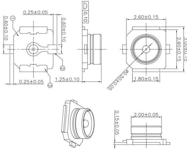
Figure 8 board end IPEX seat size diagram
