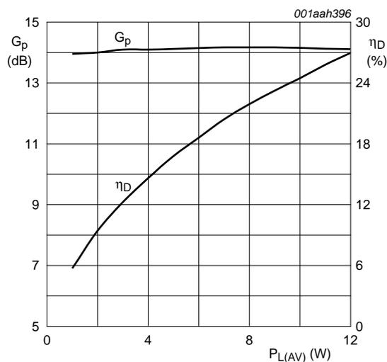
$V_{DS} = 28$  V;  $I_{Dq} = 450$  mA;  $f = 3500$  MHz.
