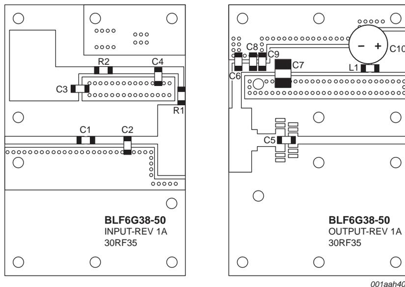
Striplines are on a double copper-clad Taconic RF35 Printed-Circuit Board (PCB) with  $\epsilon_r = 3.5$  and thickness = 0.76 mm. See [Table 9](#) for list of components.
