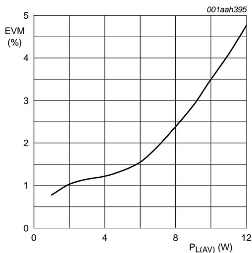
$V_{DS} = 28$  V;  $I_{Dq} = 450$  mA;  $f = 3500$  MHz.
