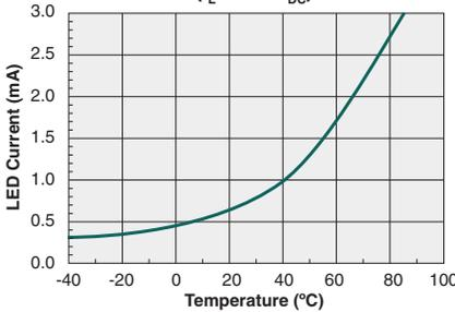
**Typical  $I_F$  for Switch Dropout vs. Temperature**
