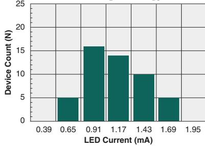
**Typical  $I_F$  for Switch Dropout**
