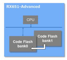
Figure 3: Dual Bank flash function
