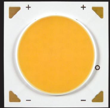
The V Series™ LED Array products deliver high quality light in a compact and cost-effective solid-state lighting package. These Chip-on-Board (CoB) arrays can be efficiently driven at twice the nominal drive current, enabling design flexibility not previously possible. This high flux density light source is designed to support a wide range of high quality, low cost directional luminaires and replacement lamps for commercial and residential applications.
