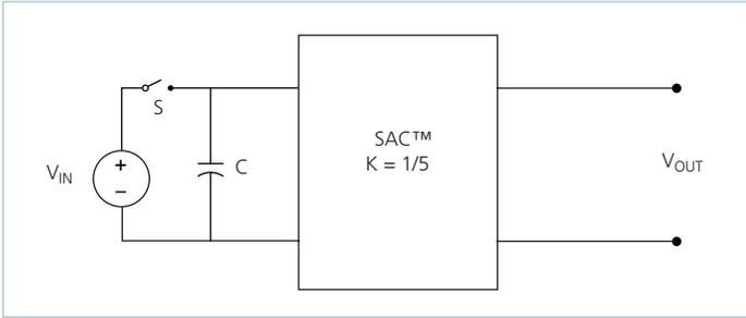
Figure 18 — Sine Amplitude Converter™ with input capacitor
