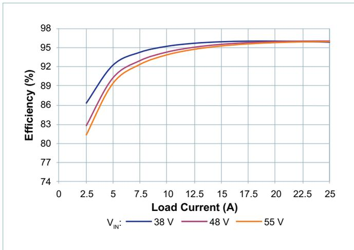
Figure 6 — Efficiency at  $T_{CASE} = 25^{\circ}C$
