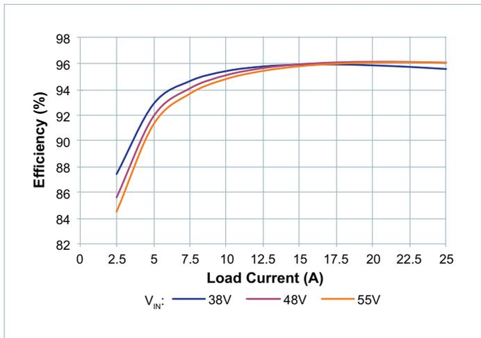
Figure 8 — Efficiency at  $T_{CASE} = 100^{\circ}C$
