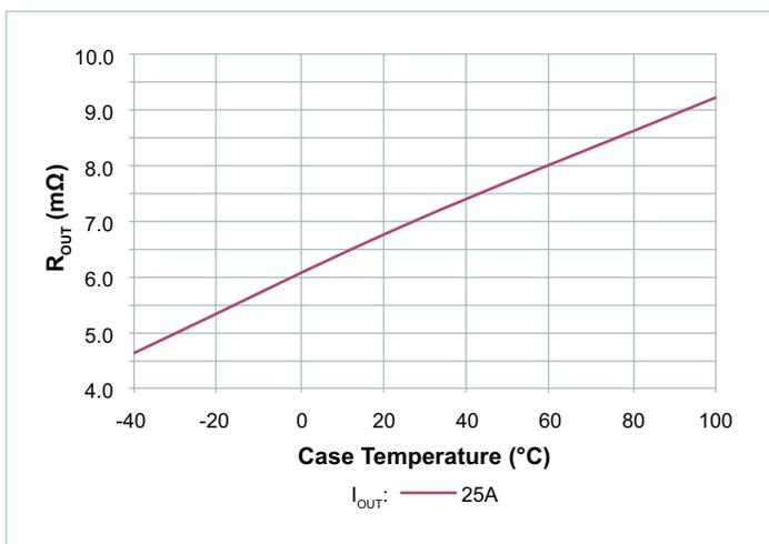
Figure 10 —  $R_{OUT}$  vs. temperature; nominal input
