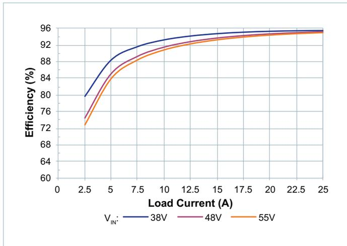
Figure 4 — Efficiency at  $T_{CASE} = -40^{\circ}C$
