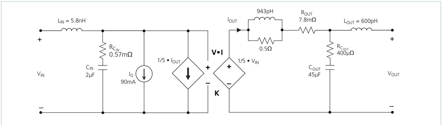
Figure 16 — VI Chip® module AC model
