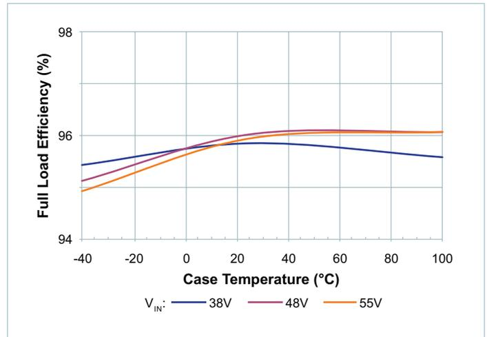
Figure 3 — Full load efficiency vs. temperature;  $V_{IN}$
