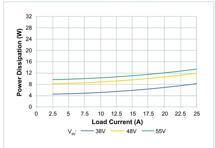
Figure 5 — Power dissipation at  $T_{CASE} = -40^{\circ}C$
