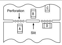
\*1 A > D is valid when stress is added vertically to the perforation as with Hand Separation. If a Cutting Disc is used, stress will be diagonal to the PCB, therefore A > D is invalid.
