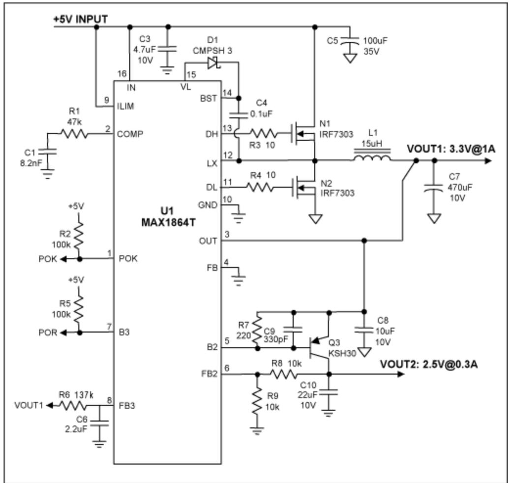
Figure 1. Two output with POR function.
