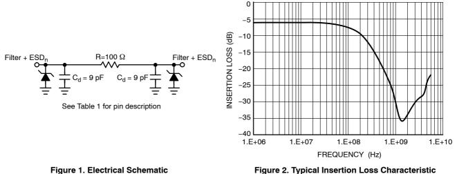
Figure 2. Typical Insertion Loss Characteristic
