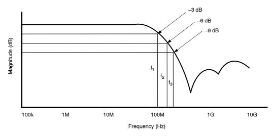
Figure 8. Filter Bandwidth
