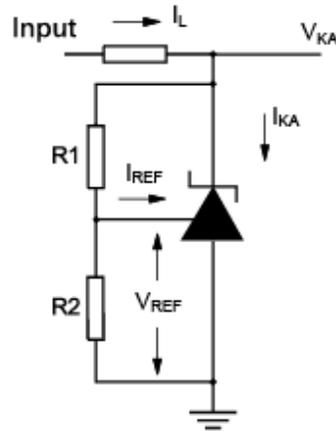
Figure 2. Test circuit for  $V_{KA} > V_{REF}$
