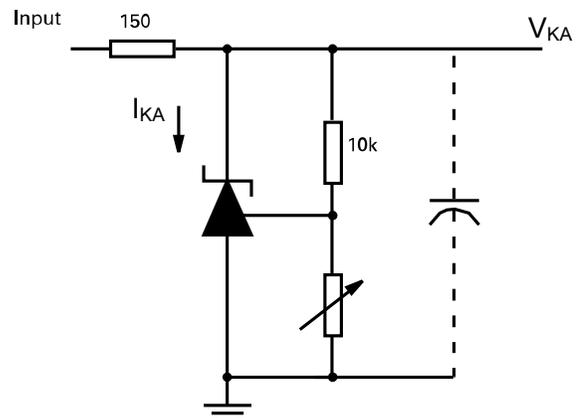
$V_{REF} < V_{KA} < 20\text{V}$ ,  $I_{KA} = 10\text{mA}$ ,  $T_A = +25^\circ\text{C}$
