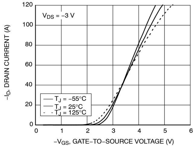
Figure 2. Transfer Characteristics
