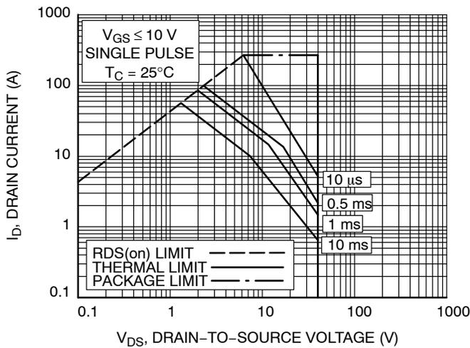
Figure 11. Maximum Rated Forward Biased Dafe operating Area
