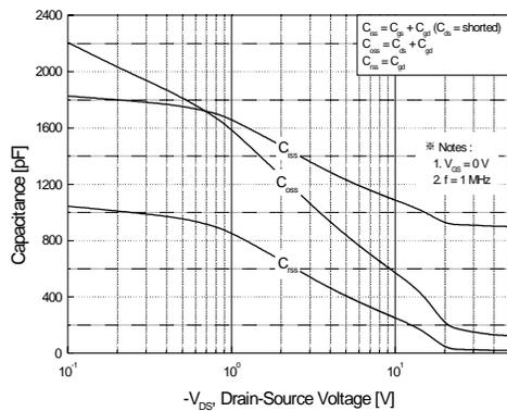
Figure 5. Capacitance Characteristics
