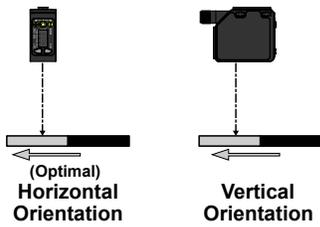
Figure 10. Orientation for highly reflective target <sup>¶</sup>
