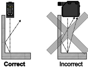
Figure 7. Orientation for a moving object
