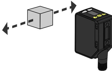
See the following figures for examples of correct and incorrect sensor-to-target orientation as certain placements may pose problems for sensing some targets. The Q5X can be used in the less preferred orientation and at steep angles of incidence and still provide reliable detection performance due to its high excess gain. For the minimum object separation distance required for each case, refer to .
