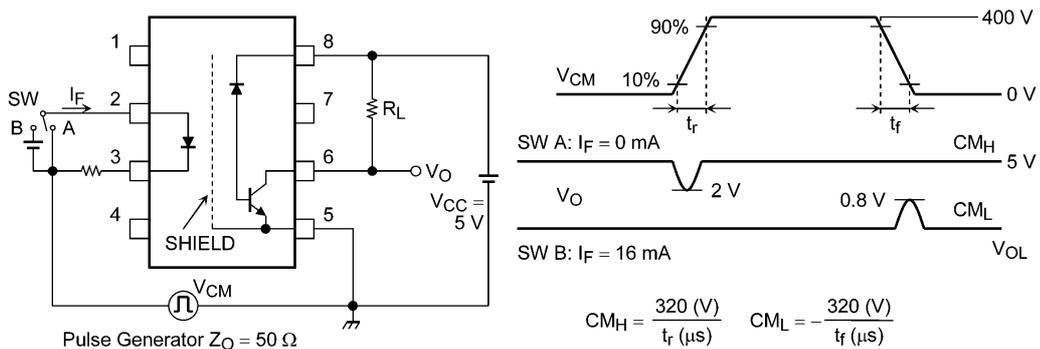
**Fig. 12.1.2 Common-Mode Transient Immunity Test Circuit and Waveform**
